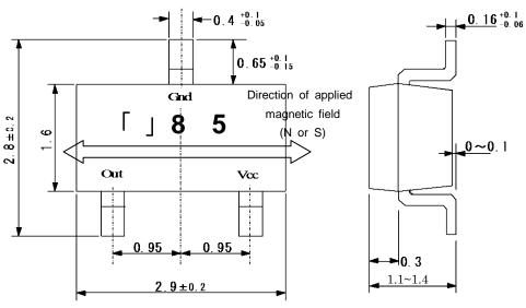
Coplanarity: less than 0.1mm(includiong under reflow condition)
