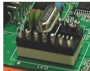
Figure 2-3. Oscillator Shape
