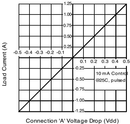
Figure 3. Linearity Characteristics
