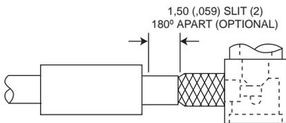
2. Insert trimmed cable into back end of body. The tubular body extension will slide under the braid with the rear portion of extension fitting under the jacket as shown. The center conductor will extend into slot in contact. NOTE: On smaller diameter cables, two longitudinal slits in the jacket, 180° apart, may be cut to ease assembly.
