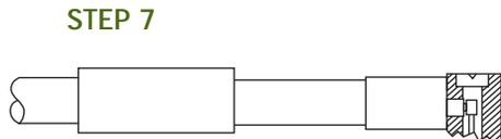
7. Locate the cap in rear of body and dimple or lightly punch to ensure it is locked in position.
