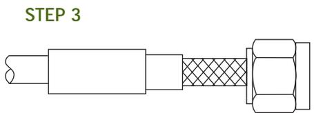
3. Insert trimmed cable into the rear of the body assembly. Tubular body extension will slide under the braid with the rear portion of extension fitting under the jacket as shown. NOTE: When using cables with inflexible jackets it is permissible to make two 3,17 (.125) long longitudinal slits in the outer jacket.
