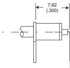
4. Bend center conductor to dimension shown depending upon preferred orientation. These dimensions suit 2,54 (.100) and 7,62 (.300) PCB pitches. For other pitches of 2,54 (.100) multiples add 2,54 (.100) multiples to the 12,70 (.500) and 6,35 (.250) dimensions in the cable stripping instructions Note 1.
