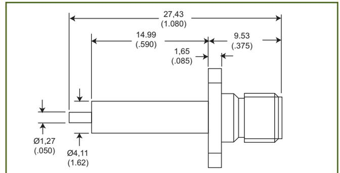
Straight Jack, Solder Pot Contact, Flush Dielectric
