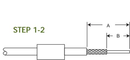
1. Slide ferrule and heat shrinkable tubing on to cable.
