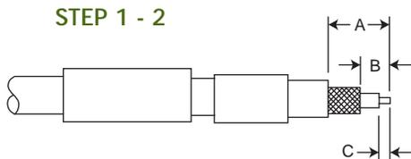
1. Slide ferrule and (if supplied) heat shrinkable tubing on to cable.
