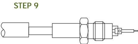
10. Insert crimped assembly into back end of body and tighten to a torque of 0.70 - 0.80 Nm (100-110 in. ozs.).
