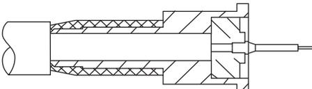
4. Place a 0,38 (.015) dia. X 2,50 +/- 0,51 (.100 +/- .020) long solder wire into solder hole of the center contact. Heat center contact and push it over cable inner conductor until it bottoms against insulator as shown. Remove excess solder if necessary.
