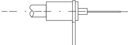
3. Slide tab-ferrule over braids to face of flange and crimp using Cannon's Crimp Tool and suitable Die Set (see table).
