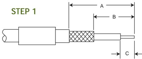
1. Trim cable to dimensions shown being careful not to nick the braid or center conductor. Tin center conductor, (DO NOT OVER TIN) then slip ferrule (and shrink tubing if supplied) over cable.
