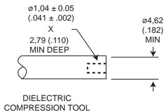
5. Compress expanded dielectric back into cable outer conductor with Dielectric Compression Tool as shown, until it is flush with end of body and outer conductor.
