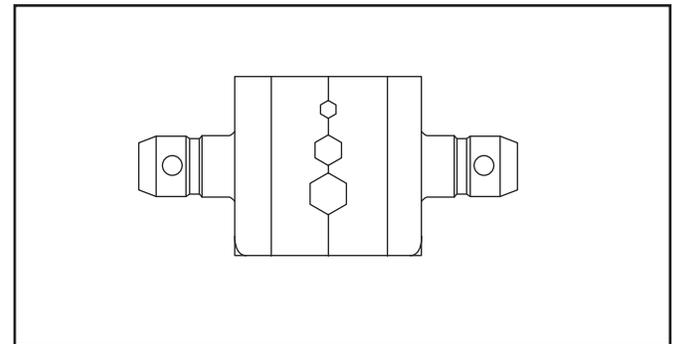
Torque Wrench (for SMA coupling nut - mating)
