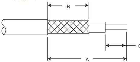
1. Strip cable to dimensions shown. Do not nick outer or inner conductors. Tin inner conductor.
