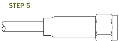
5. Slide heat shrinkable tubing over ferrule and apply heat until tubing shrinks down.
