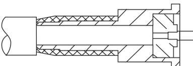
3. Insert cable dielectric into rear body until it bottoms firmly against insulator as shown.
