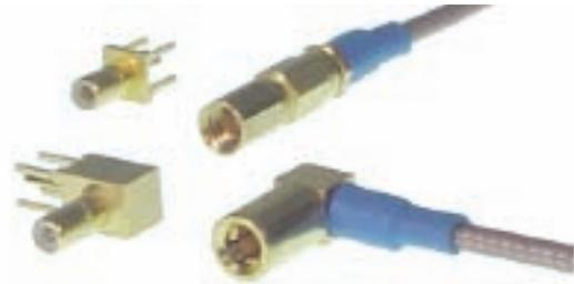
SSMC connectors are used where a positive mechanical engagement is required and where space permits the use of torque wrenches. SSMB connectors are quick disconnect versions of the SSMC and are used in applications where limited space prohibits the use of torque wrenches or when components or modules must be quickly changed to keep down time to a minimum.
