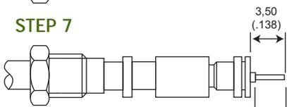
7. Trim cable dielectric and center conductor to dimensions shown taking care not to nick the center conductor.
