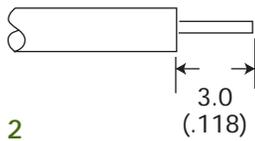
1. Remove cable outer conductor and dielectric to the dimension shown, being careful not to fracture the center conductor. Tin center conductor (DO NOT OVER TIN).
