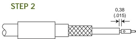
2. Solder center conductor to contact. With AI-102 and AI-236 the gap shown is to be maintained.
