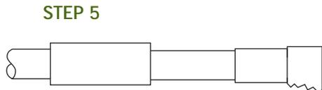
4. Slide body over cable dielectric and under the braid until braid is flush against underside of body. Ensure center conductor is located in the forked end of the contact. NOTE: When using cables with inflexible jackets it is permissible to make two 3,17 (.125) longitudinal slits in the outer jacket.
