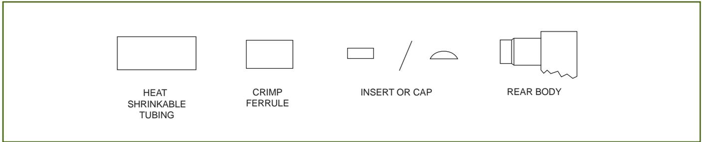
1. Slide heat shrinkable tubing and ferrule on to cable.
