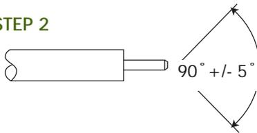
2. Point the end of the center conductor using a miniature file or suitable tool.
