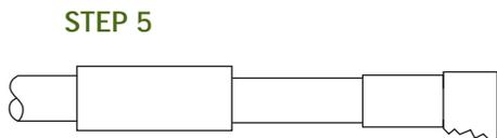
5. Slide ferrule flush against the body and crimp in position using Cannon's Crimp Tool and suitable Die Set (see table).
