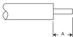
1. Cut cable end square. Remove the cable outer conductor and dielectric to the dimension shown taking care not to nick the center conductor. Deburr outer conductor at point of cut.
