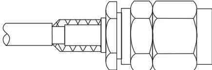
5. Insert rear body into front body. Engage threads of retaining nut to front body and hand tighten retaining nut. Hold front body firmly with a 7,93 (.312) hex. torque wrench and torque it to 1,13 - 1,69 Nm (10-15 in. lbs) by turning retaining nut only.
