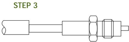
3. Slide body over cable dielectric and under the braid until the braid is flush against the rear of the hexagonal nut. NOTE: When using cables with inflexible jackets, it is permissible to make two 3,17 (.125) longitudinal slits in the outer jacket.
