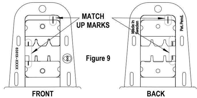
4. Do the same thing with the lower tooling and tighten the M3 screws. Be sure the small markings line up.
