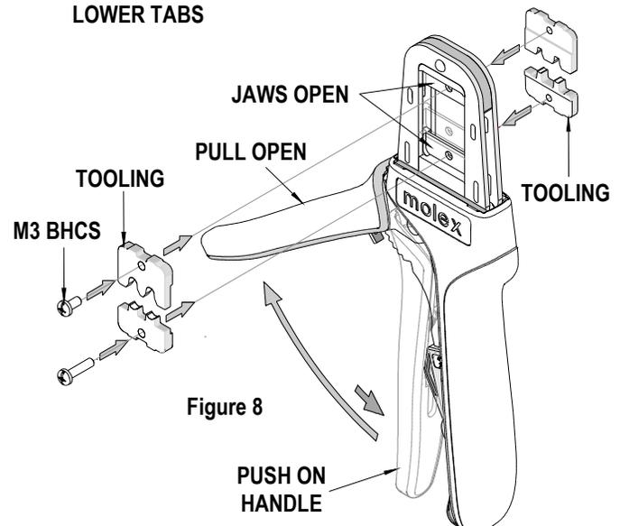
1. The locator must be removed before reversing the tooling.
