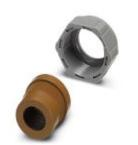
Half screw connection Pg21, made of plastic, consisting of rubber seal with one elongated hole and one pressure screw, for type 2 - 4 housings, cable diameter:  $20 \times 7$  mm
