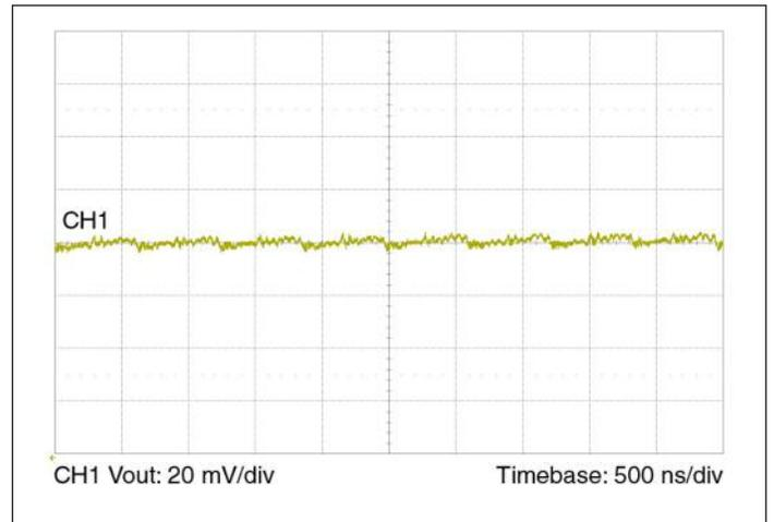
**Figure 8** — Output voltage ripple at full load and 48  $V_{IN}$  with 30  $\mu\text{F}$  ceramic external bypass capacitor and 20 nH of distribution inductance.
