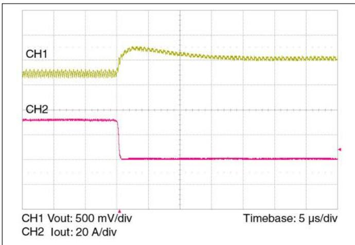
**Figure 11** — 30 – 0 A load step with 100  $\mu\text{F}$  input capacitor and no output capacitor.
