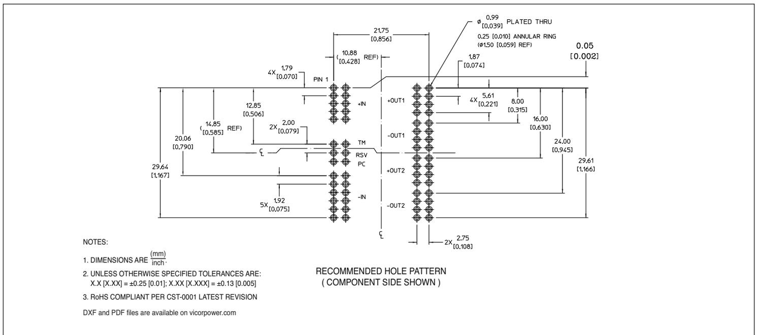
Figure 18 — BCM<sup>®</sup> through-hole module PCB layout information
