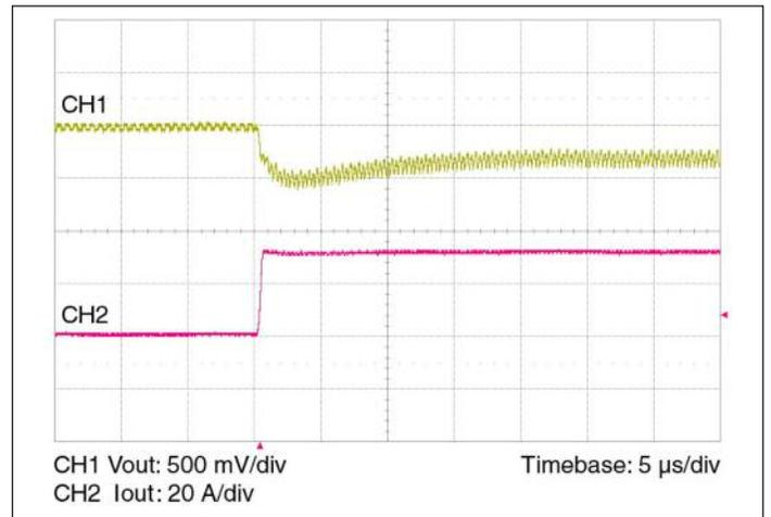
**Figure 10** — 0 – 30 A load step with 100  $\mu\text{F}$  input capacitor and no output capacitor.
