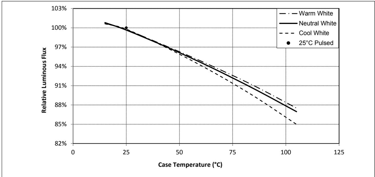
**Figure 6: Typical DC ccy Shift vs. Case Temperature**
