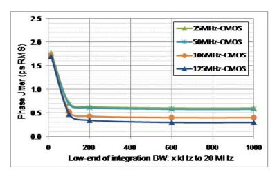
Figure 1. LVCMOS Phase Jitter (integrated phase noise)
