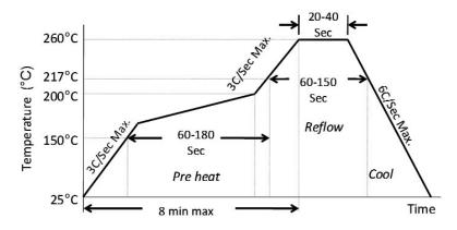
Figure 3. Solder Reflow Profile
