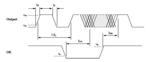
Figure 2. LVCMOS Output Waveform
