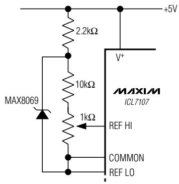
(b) Double-Regulated 100mV Reference for ICL7107 One-Chip DPM Circuit
