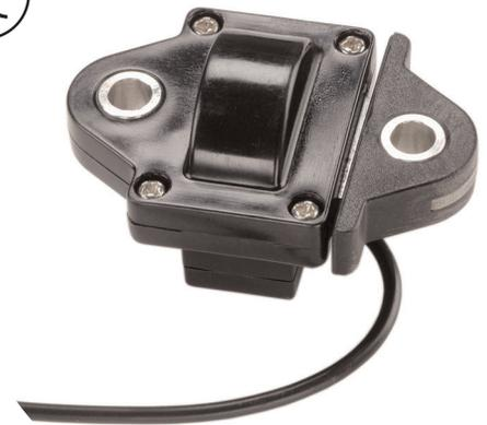
Operating at very low strains, Microfused™ technology provides gage factors greater than 100, an essentially unlimited cycle life expectancy, superior resolution, exceedingly high over-range margins without the need for stops and a ratiometric span of up to 4V. Microfused™ sensors are used in a variety of applications including bathroom scales, paint sprayers and safety-critical automotive brake sensors.
