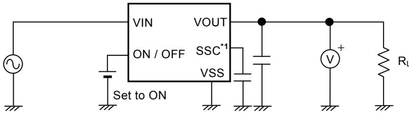
**Figure 17 Test Circuit 5**
