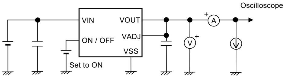
**Figure 24 Test Circuit 12**
