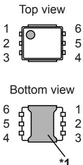
**\*1.** Connect the heatsink of backside at shadowed area to the board, and set electric potential open or GND.
