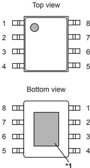
\*1. Connect the heat sink of backside at shadowed area to the board, and set electric potential GND. However, do not use it as the function of electrode.
