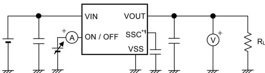
Figure 16 Test Circuit 4
