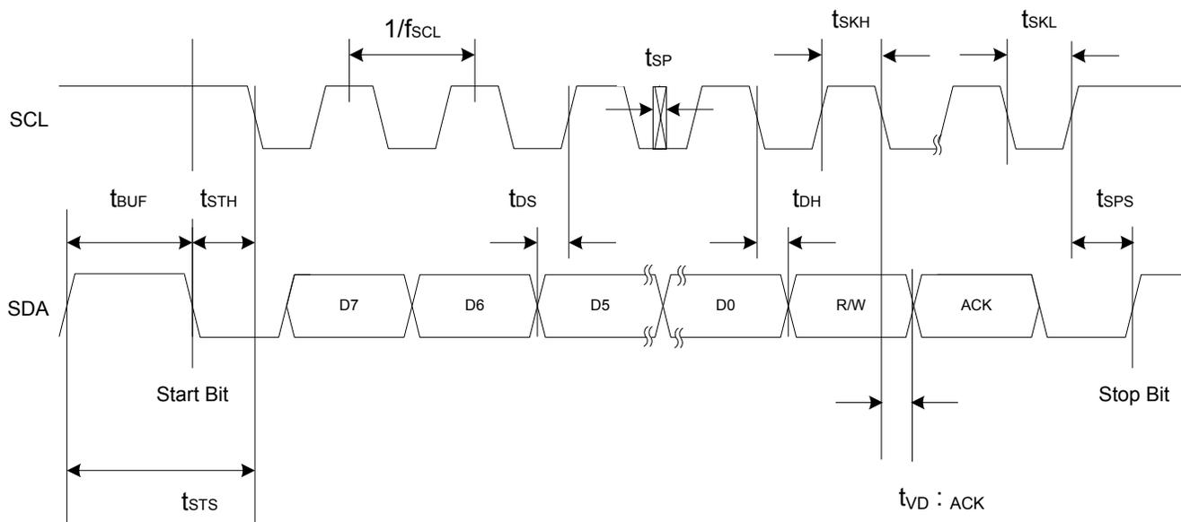
**Figure 1. I<sup>2</sup>C Interface Timing Diagram**
