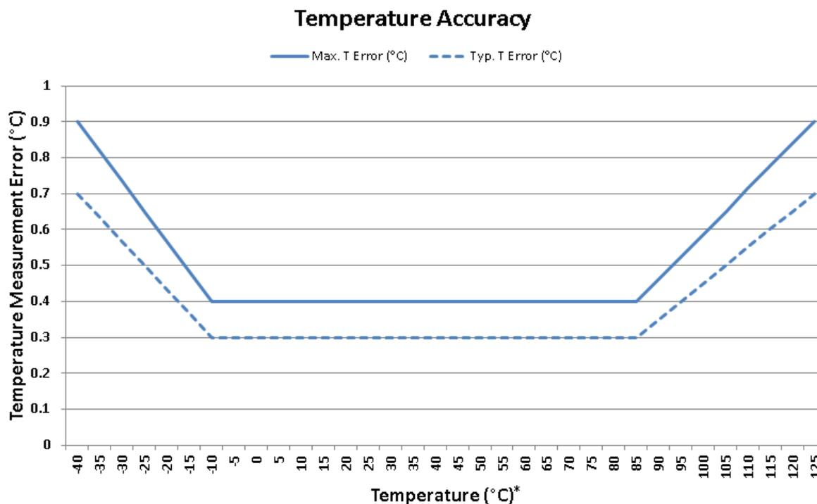
**Figure 3. Temperature Accuracy\***
