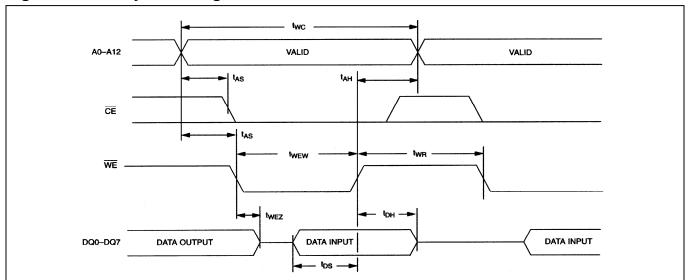
Figure 6. Write Cycle Timing, Write-Enable Controlled
