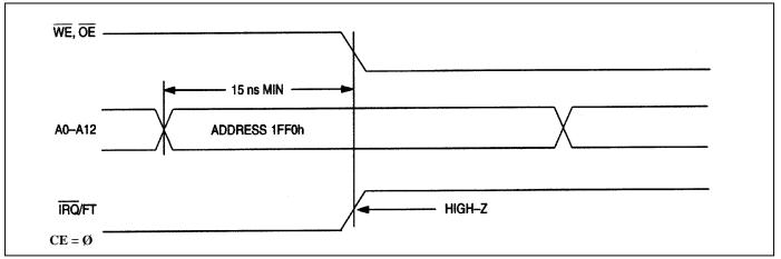
The  $\overline{IRQ}/FT$  pin can also be activated in the battery-backed mode. The  $\overline{IRQ}/FT$  goes low if an alarm occurs and both ABE and AE are set. The ABE and AE bits are cleared during the power-up transition, however, an alarm generated during power-up sets AF. Therefore, the AF bit can be read after system power-up to determine if an alarm was generated during the power-up sequence. Figure 4 illustrates alarm timing during the battery-backup mode and power-up states.
