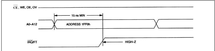
Figure 3. Clearing IRQ Waveforms
