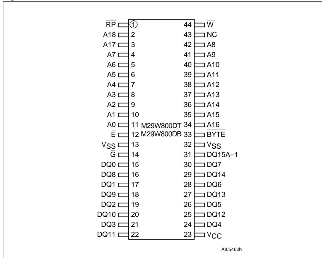
Figure 3. TSOP connections
