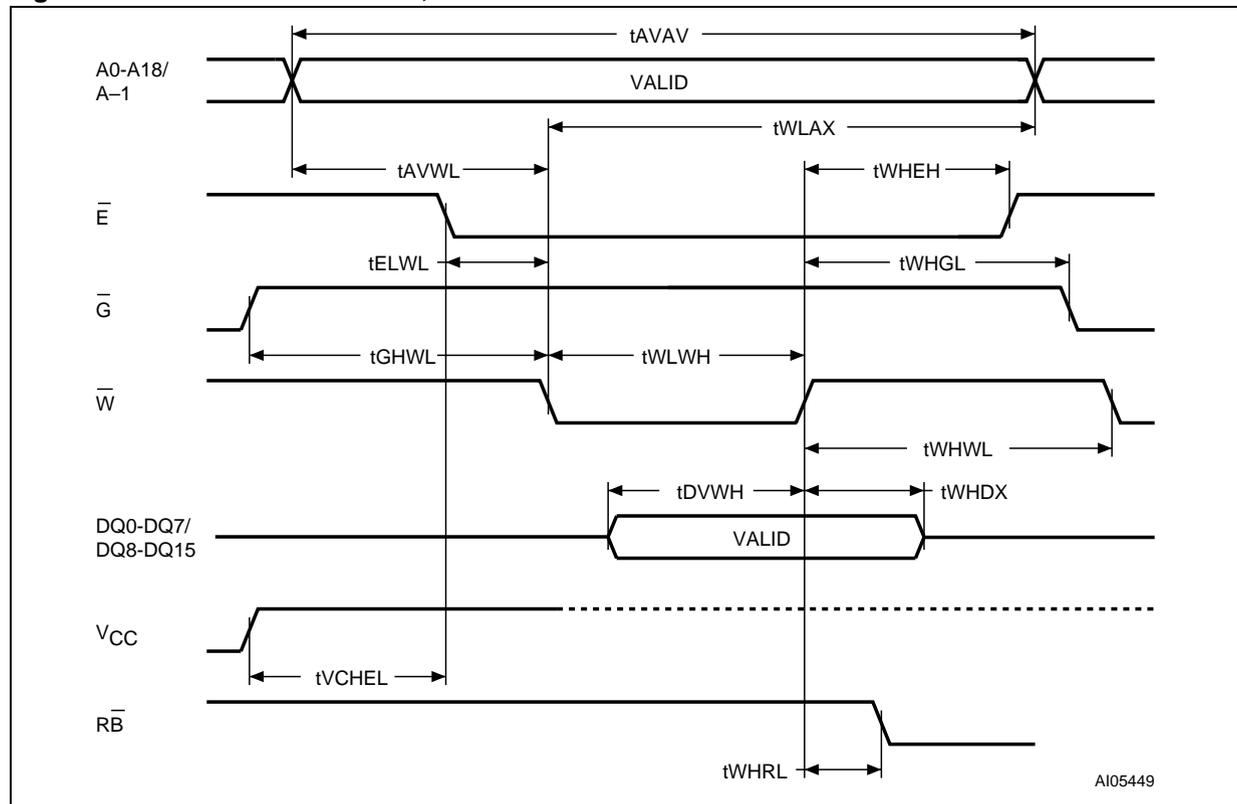
Table 13. Write AC characteristics, write enable controlled
