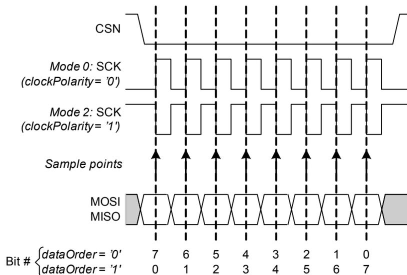
Figure 62. SPI Modes 0 and 2: clockPhase = '0'. One byte transmission.
