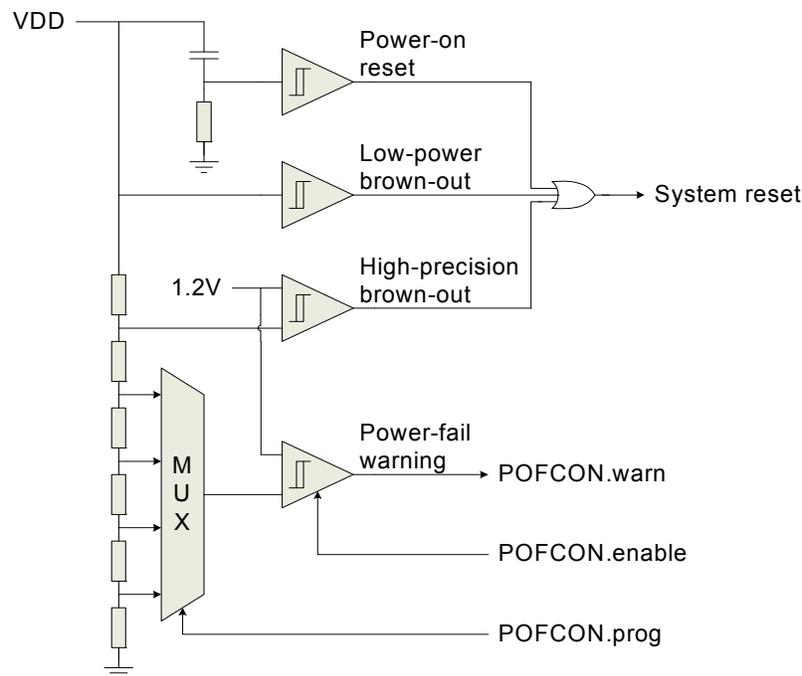
Figure 50. Block diagram of power supply supervisor
