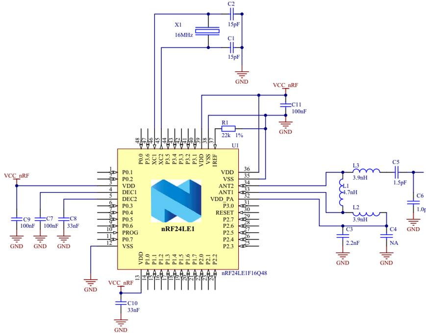
Figure 79. nRF24LE1, 7x7mm QFN48 schematic
