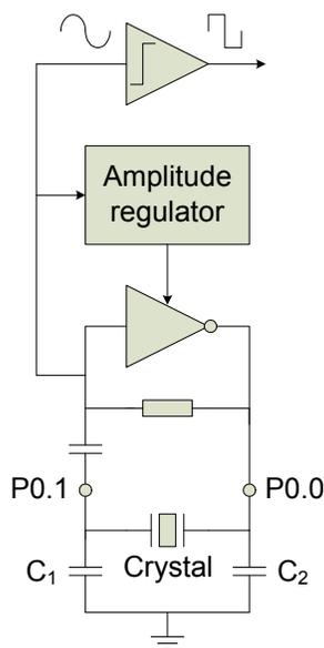
Figure 55. Block diagram of 32.768 kHz crystal oscillator
