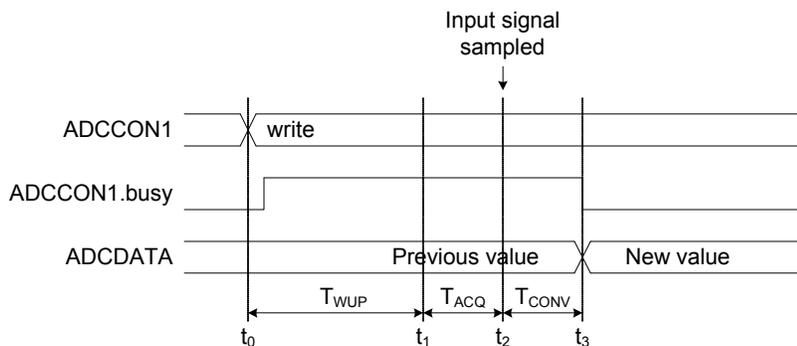
Figure 71. Timing diagram for single step conversion
