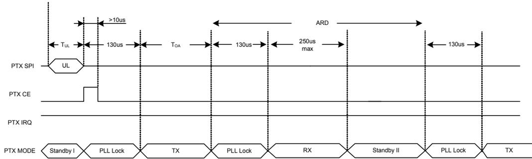
Figure 19. Timing of Enhanced ShockBurst™ when the first ACK packet is lost (2Mbps)
