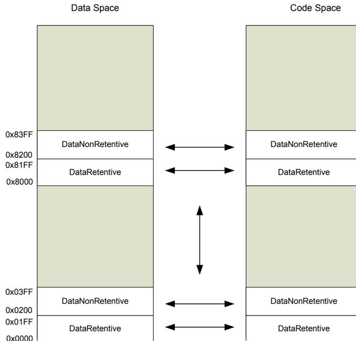
Figure 37. Configurability of SRAM address space location
