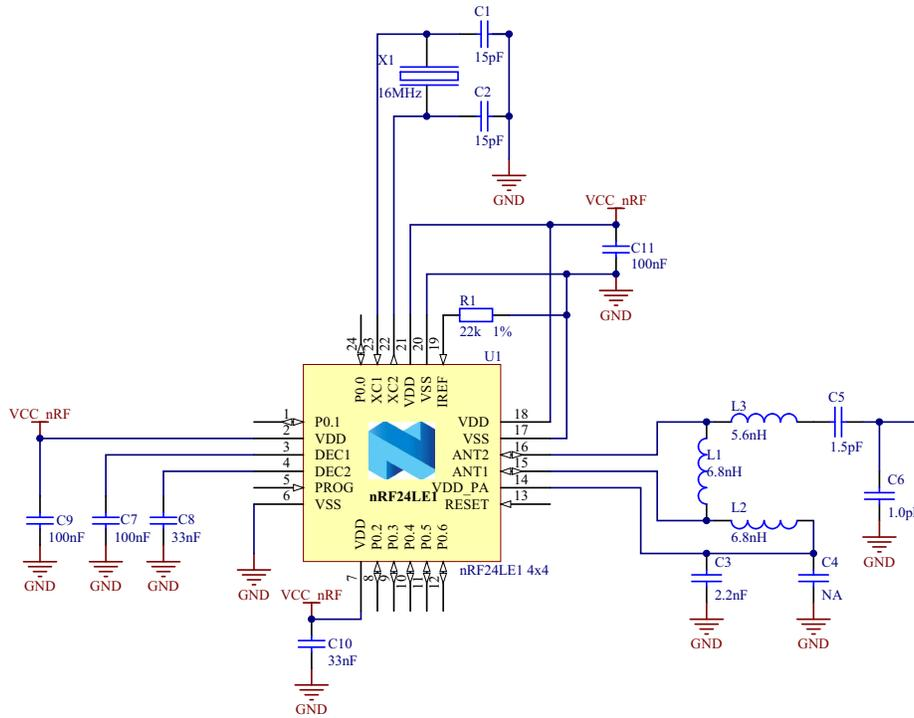
Figure 81. nRF24LE1, 4x4mm QFN24 schematic
