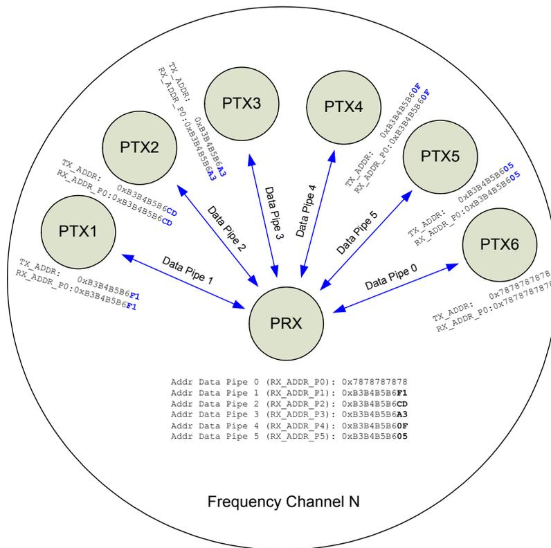
Figure 16. Example of data pipe addressing in MultiCeiver™
