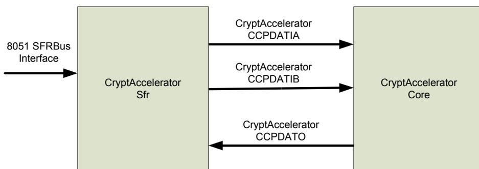
Figure 57. Encryption/decryption accelerator
