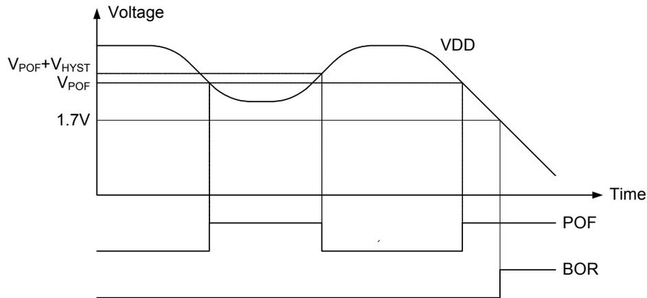
Figure 53. Power-fail comparator
