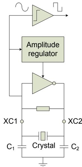
Figure 54. Block diagram of 16 MHz crystal oscillator
