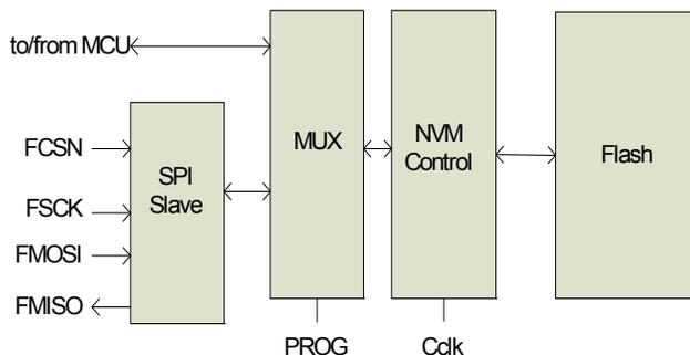
Figure 31. nRF24LE1 Flash block diagram
