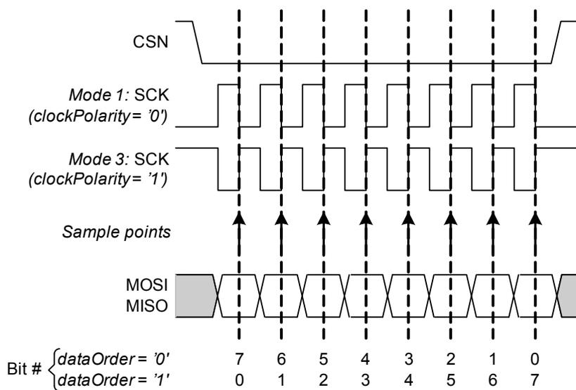
Figure 63. SPI Modes 1 and 3: clockPhase = '1'. One byte transmission.
