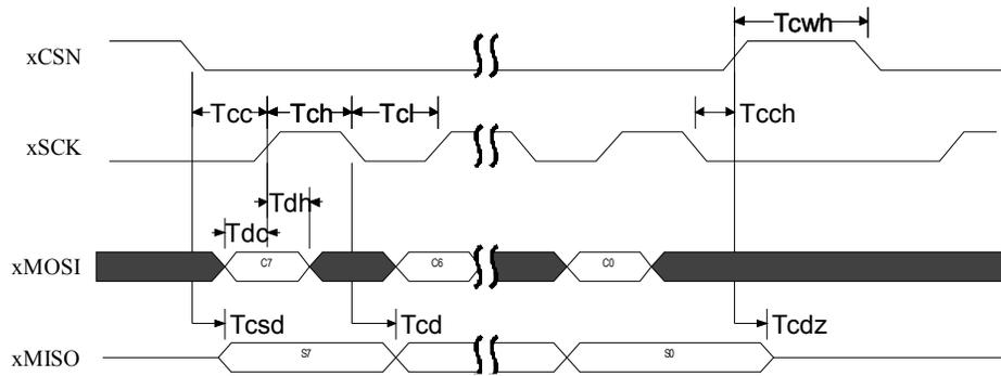
Figure 64. SPI timing diagram. One byte transmission.
