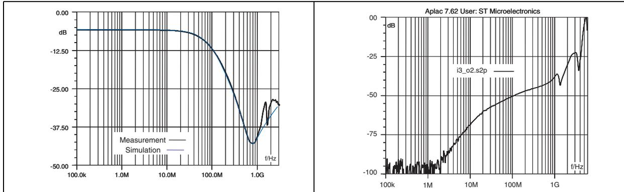
**Figure 5. Digital crosstalk measurements** **Figure 6. ESD response to IEC 61000-4-2 (+15 kV air discharge) on one input (V<sub>in</sub>) and one output (V<sub>out</sub>)**
