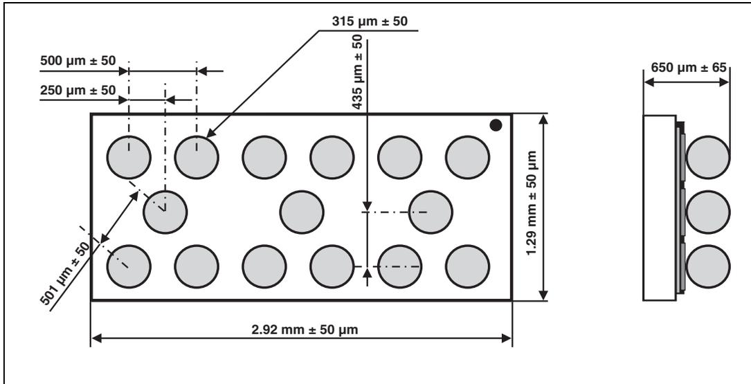
Figure 12. Foot print recommendations Figure 13. Marking
