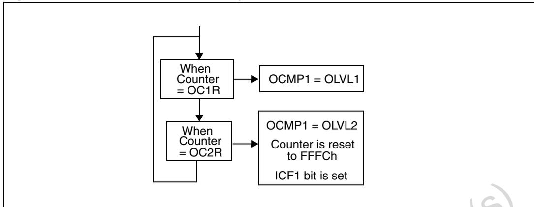
If  $OLVL1 = 1$  and  $OLVL2 = 0$  the length of the positive pulse is the difference between the  $OC2R$  and  $OC1R$  registers.
