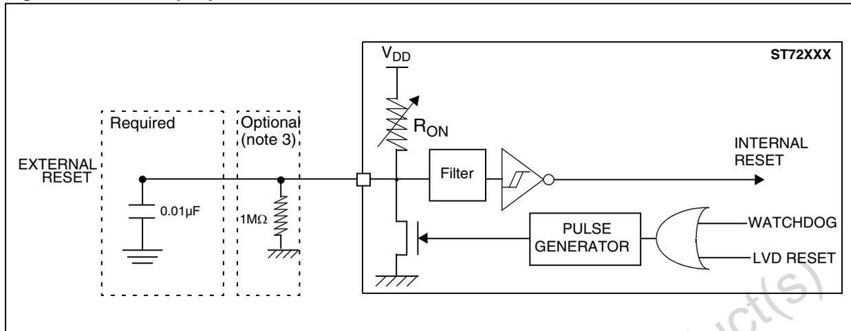
Note: 1 The reset network protects the device against parasitic resets.
