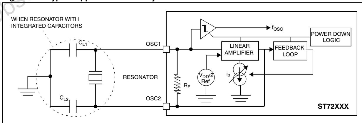
Figure 76. Application with a crystal or ceramic resonator for ROM (LQFP64 or any 48/60K ROM)
