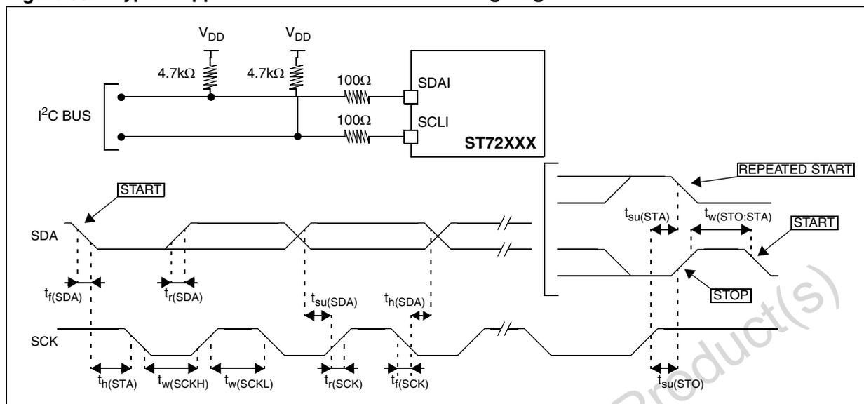
1. Measurement points are done at CMOS levels:  $0.3 \times V_{DD}$  and  $0.7 \times V_{DD}$ .
