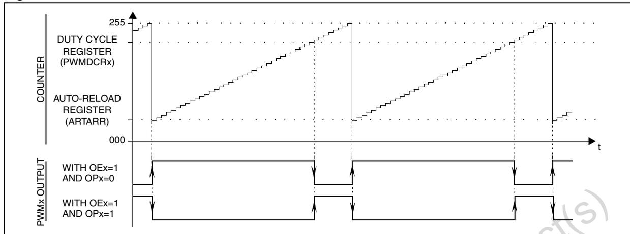
Figure 38. PWM signal from 0% to 100% duty cycle
