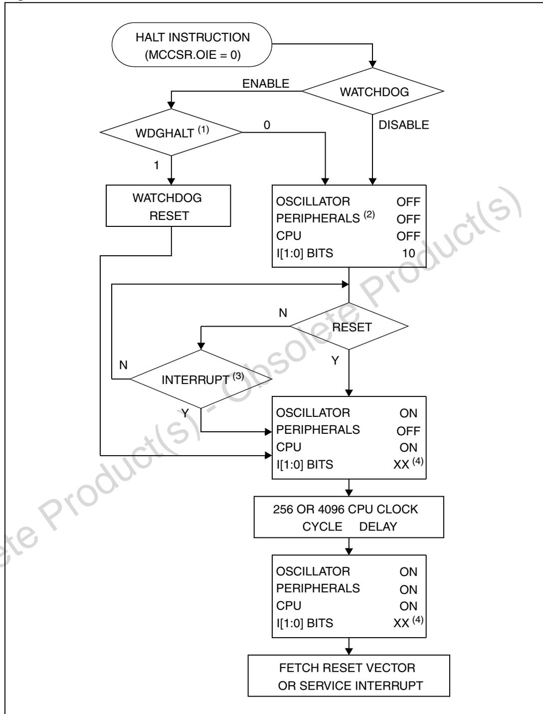
1. WDGHALT is an option bit. See [Section 21.1.1: Flash configuration on page 225](#) for more details.
