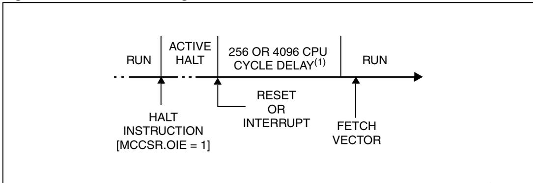
1. This delay occurs only if the MCU exits Active Halt mode by means of a RESET.
