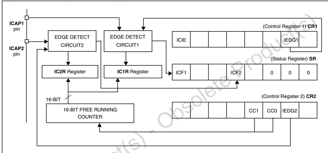
Figure 47. Input capture timing diagram
