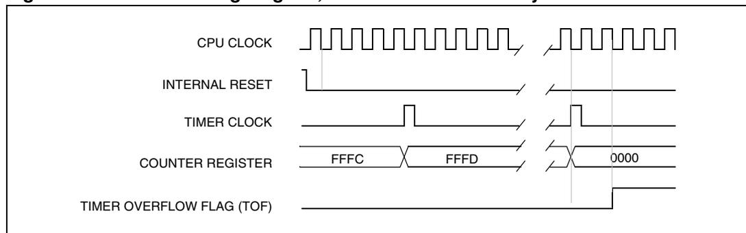
*Note:* The MCU is in reset state when the internal reset signal is high; when it is low the MCU is running.
