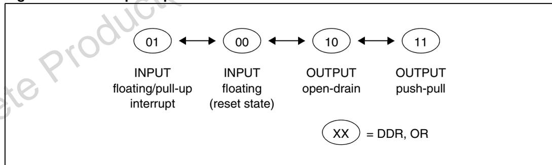
The I/O port register configurations are summarized in the following table.
