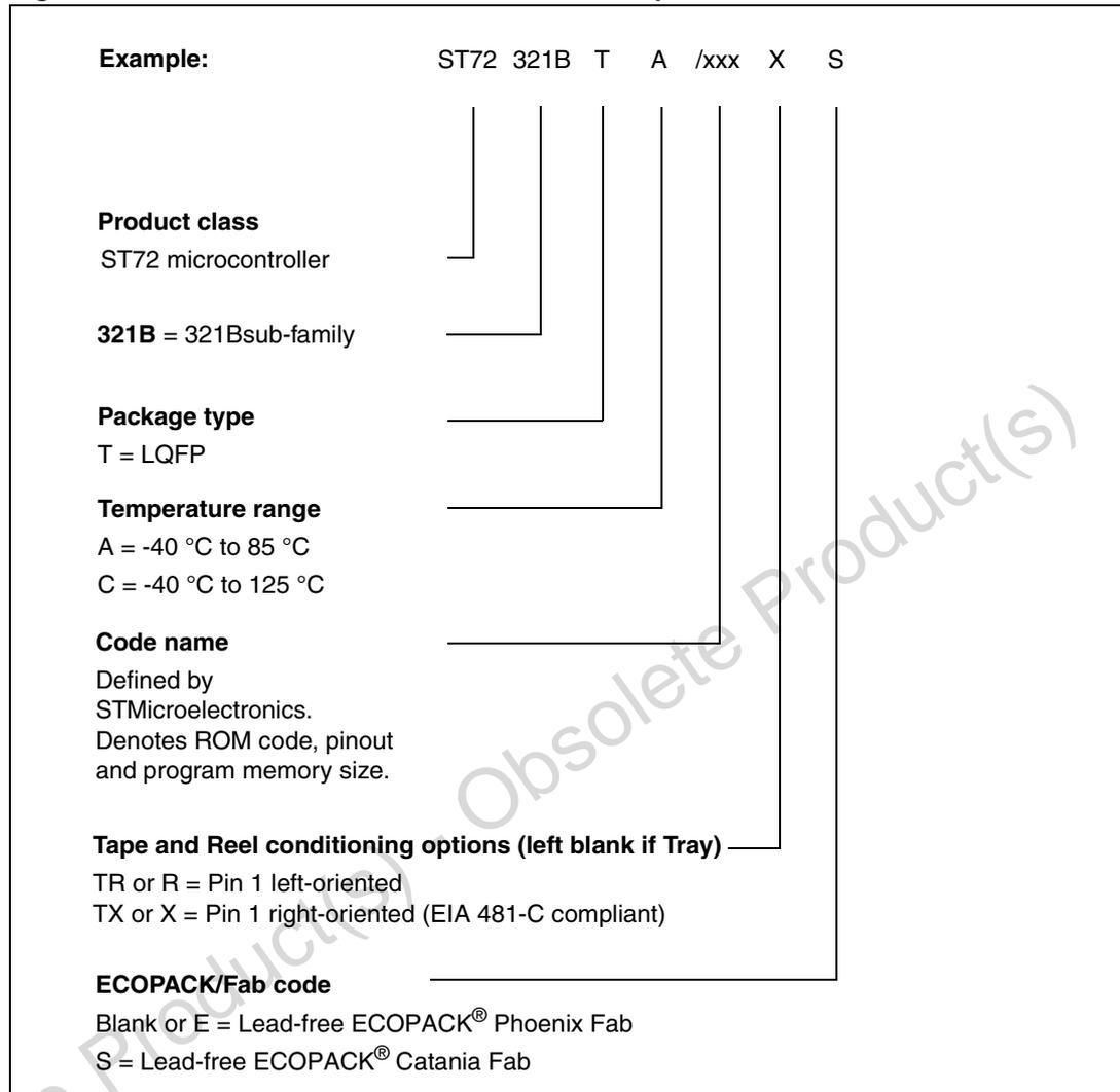
**Figure 106. ST72321B-Auto microcontroller FASTROM/ROM option list**
