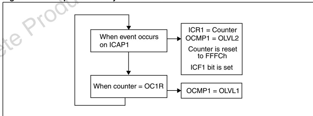
Because the ICF1 bit is set when an active edge occurs, an interrupt can be generated if the ICIE bit is set.
