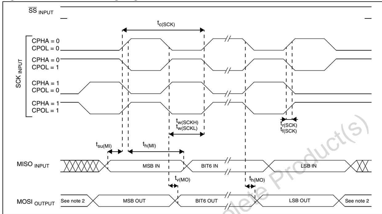
1. Measurement points are done at CMOS levels:  $0.3 \times V_{DD}$  and  $0.7 \times V_{DD}$ .
