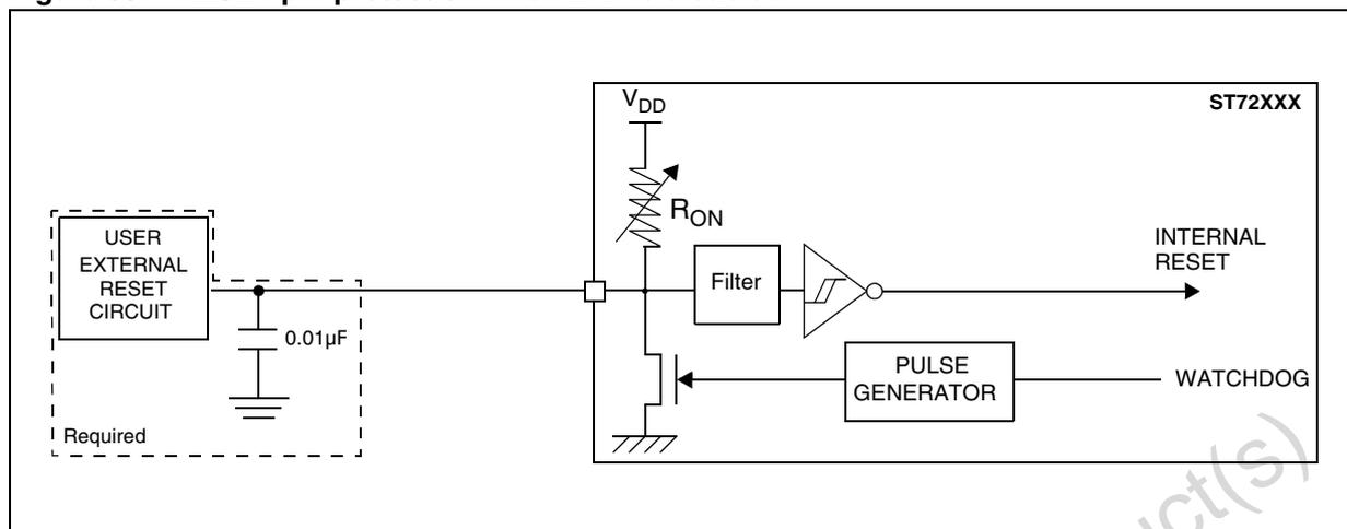
**Note:** The reset network protects the device against parasitic resets. The output of the external reset circuit must have an open-drain output to drive the ST7 reset pad. Otherwise the device can be damaged when the ST7 generates an internal reset (LVD or watchdog).
