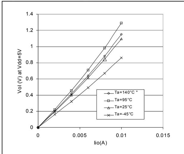
Figure 82. Typical  $V_{OL}$  at  $V_{DD} = 5V$  (high-sink)
