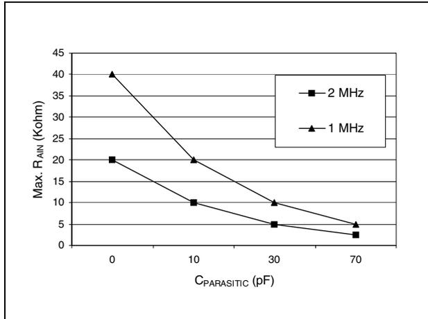
1.  $C_{PARASITIC}$  represents the capacitance of the PCB (dependent on soldering and PCB layout quality) plus the pad capacitance (3pF). A high  $C_{PARASITIC}$  value will downgrade conversion accuracy. To remedy this,  $f_{ADC}$  should be reduced.
