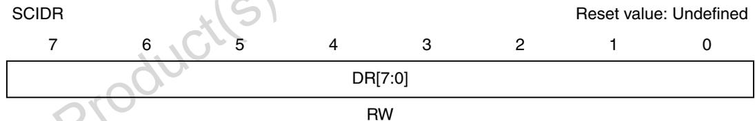
The Data register performs a double function (read and write) since it is composed of two registers, one for transmission (TDR) and one for reception (RDR).
