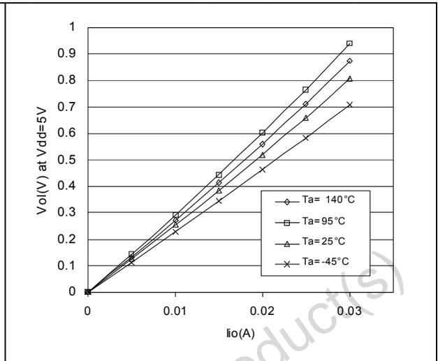
Figure 83. Typical  $V_{OH}$  at  $V_{DD} = 5V$
