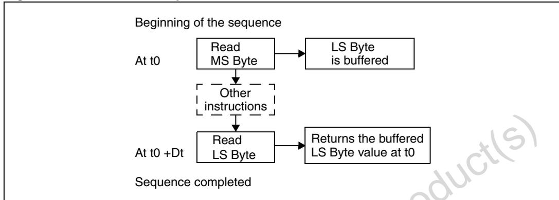
The user must read the MS Byte first; the LS Byte value is then buffered automatically.
