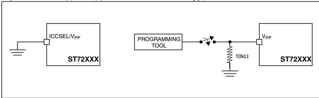
1. When ICC mode is not required by the application, the ICCSEL/V<sub>PP</sub> pin must be tied to V<sub>SS</sub>.
