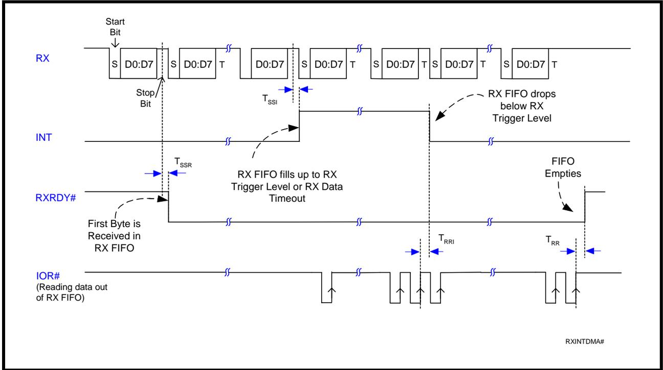
**FIGURE 20. RECEIVE READY & INTERRUPT TIMING [FIFO MODE, DMA ENABLED] FOR CHANNELS A & B**
