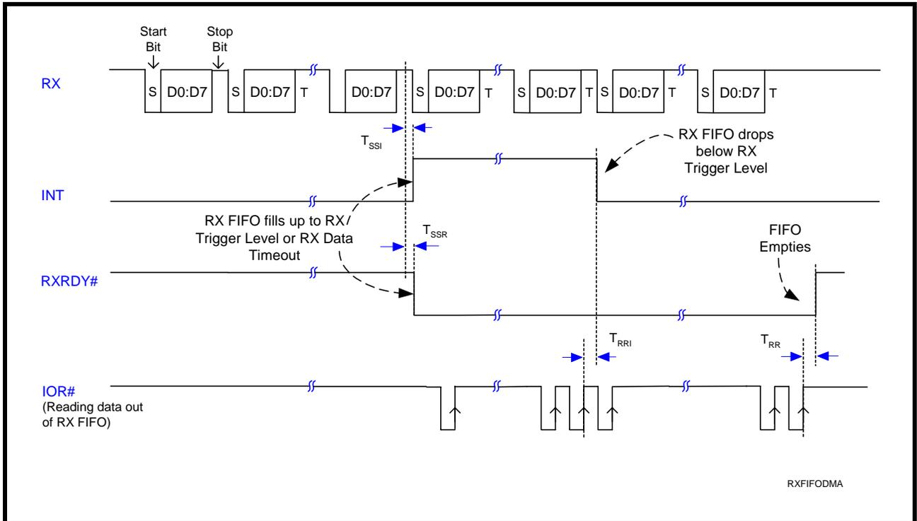
FIGURE 21. TRANSMIT READY & INTERRUPT TIMING [FIFO MODE, DMA MODE DISABLED] FOR CHANNELS A & B
