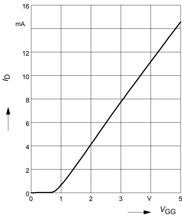
**Drain current  $I_D = f(V_{G1S})$**
