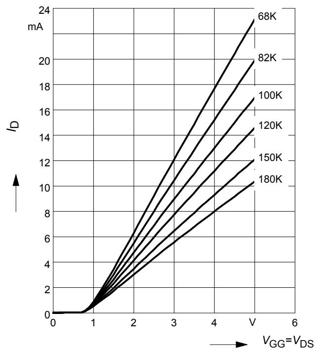
**Drain current  $I_D = f(V_{G2S})$**
