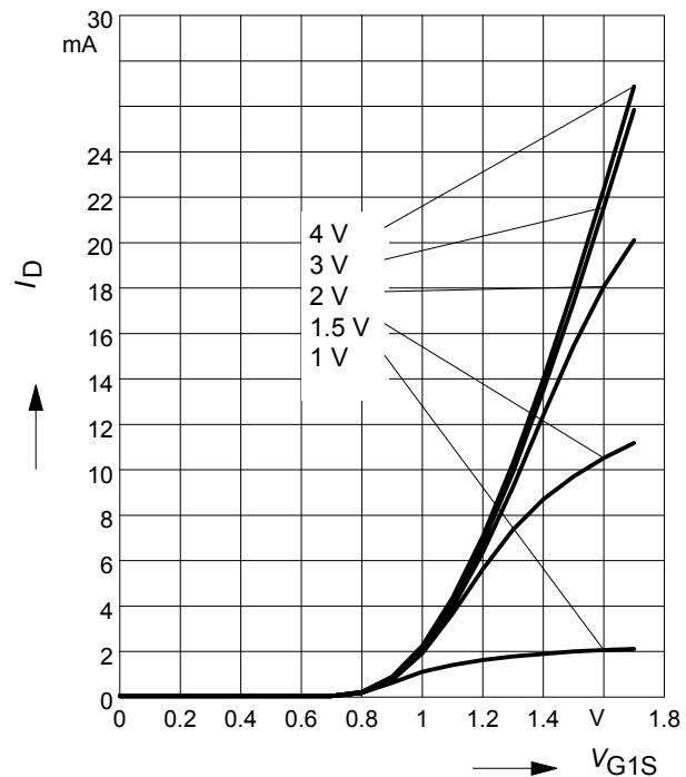
**Drain current  $I_D = f(V_{GG})$**
