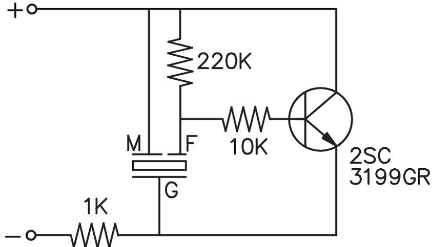
Notes: 1. The current consumption and the sound pressure level are measured by using the recommend driving circuit shown above.
