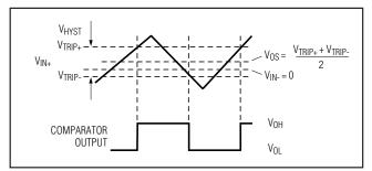
Figure 1. Input and Output Waveforms, Noninverting Input Varied
