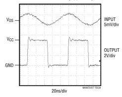
**10MHz RESPONSE** HIGH-SPEED MODE ( $V_{CC} = +3V$ )
