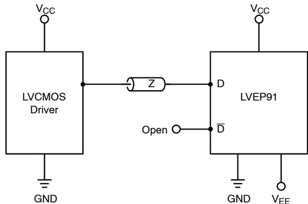
Figure 11. Standard LVCMOS Interface ( $\bar{D}$  will default to  $V_{CC}/2$  when left open. A reference voltage of  $V_{CC}/2$  should be applied to D input, if  $\bar{D}$  is interfaced to CMOS signals.)
