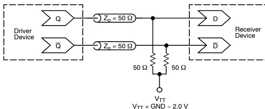
**Figure 12. Typical Termination for Output Driver and Device Evaluation
