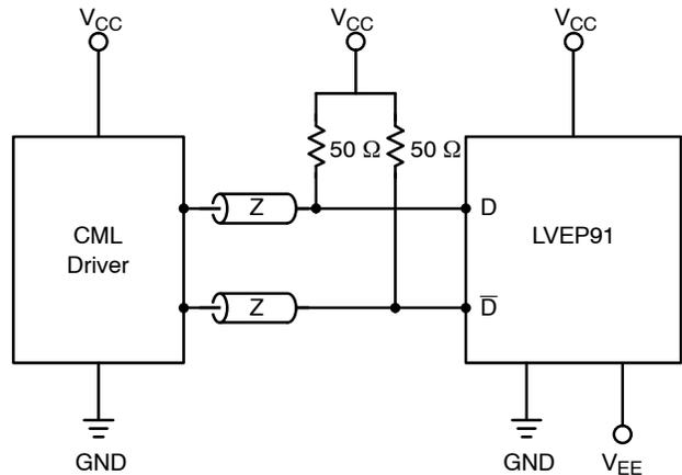
Figure 9. Standard 50  $\Omega$  Load CML Interface
