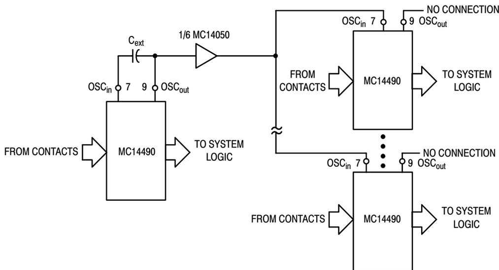
Figure 5. Typical Single Oscillator Debounce System
