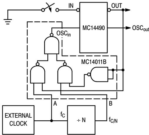
Figure 6. Fast Attack/Slow Release Circuit
