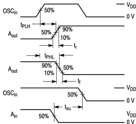
Figure 1. Switching Waveforms
