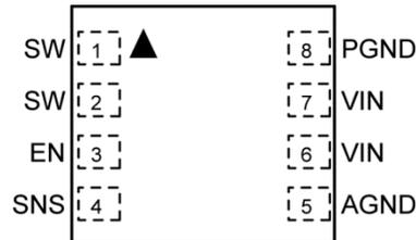
8-Pin 2mm x 2mm Thin DFN (MM)
