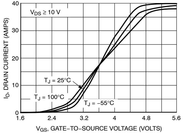
**Figure 2. Transfer Characteristics**
