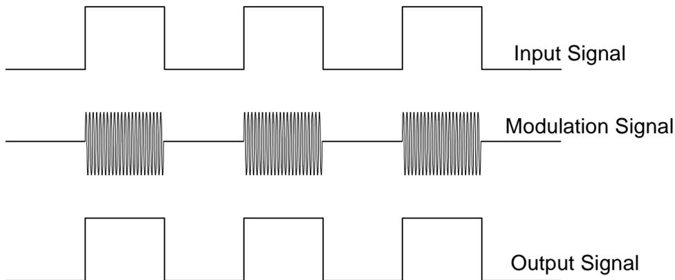
**Figure 10. Modulation Scheme**
