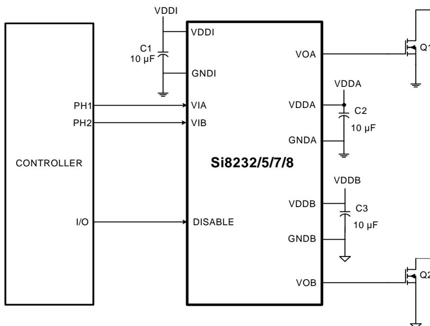
**Figure 44. Si8232/5/7/8 in a Dual Driver Application**
