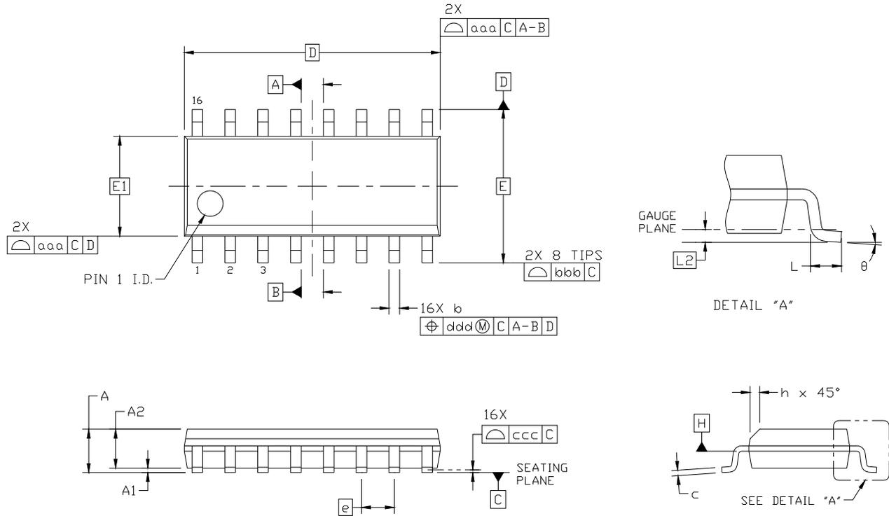
**Figure 47. 16-pin Small Outline Integrated Circuit (SOIC) Package**
