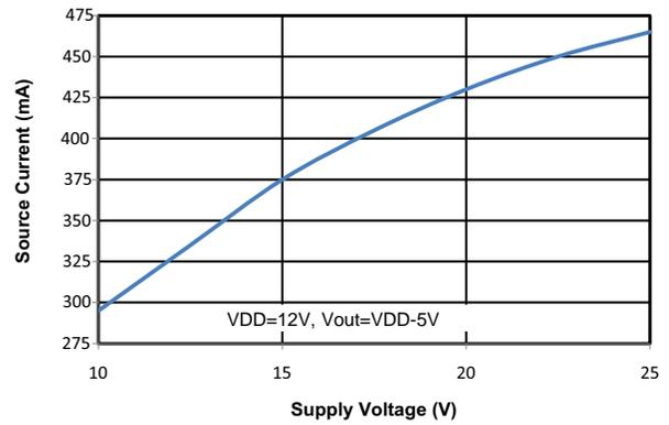
**Figure 20. Output Source Current vs. Supply Voltage**
