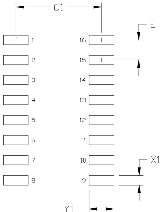
**Figure 48. 16-Pin Narrow Body SOIC PCB Land Pattern**
