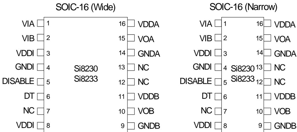
**Table 11. Si8230/3 Two-Input HS/LS Isolated Driver (SOIC-16)**
