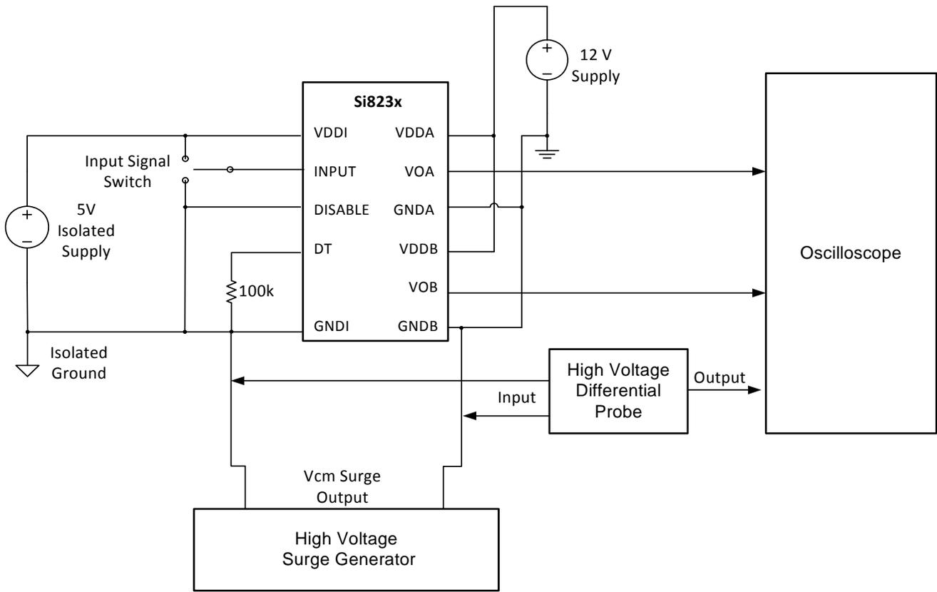
**Figure 6. Common Mode Transient Immunity Test Circuit**
