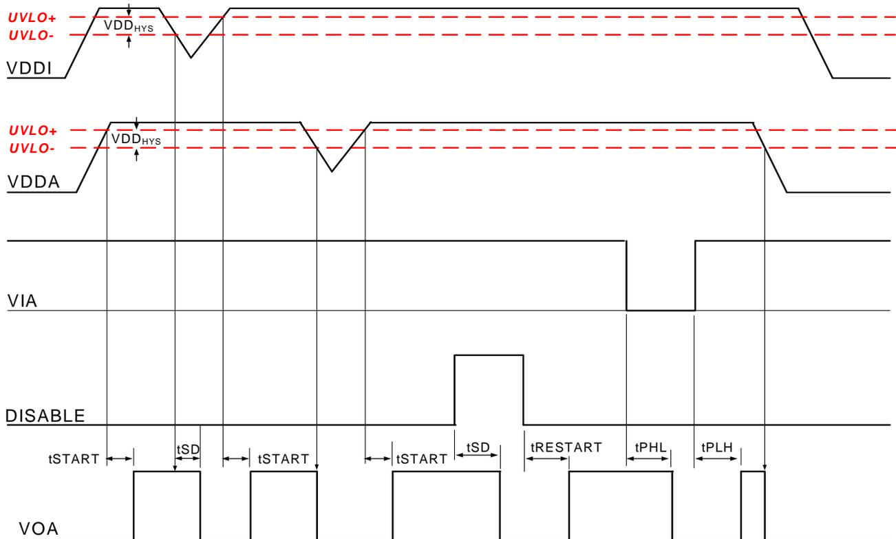
Figure 36. Device Behavior during Normal Operation and Shutdown
