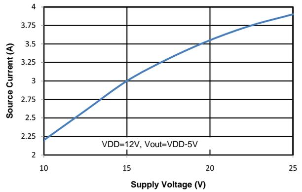
Figure 32. Output Source Current vs. Supply Voltage
