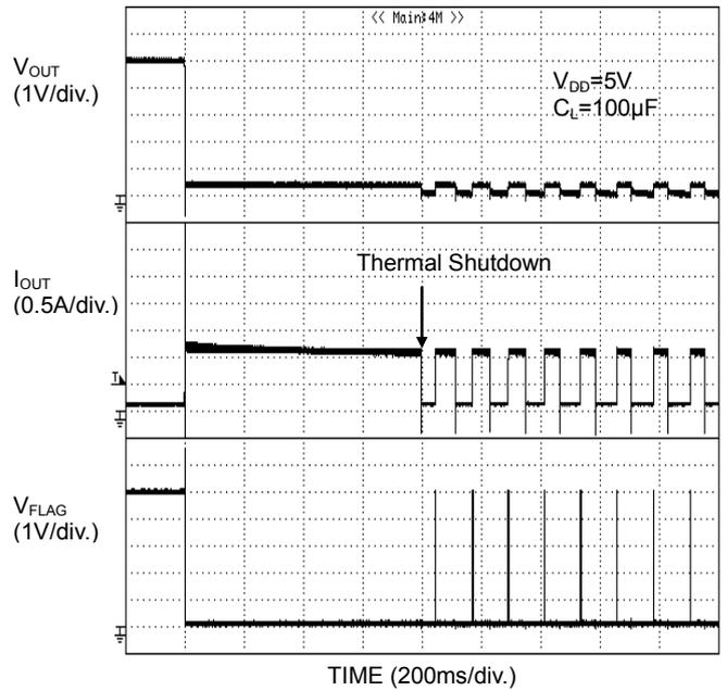
Figure 34. Over-Current Response Output Short Circuit at Enable
