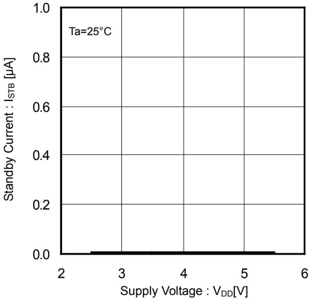
Figure 5. Standby Current vs Supply Voltage (CTRL Disable)
