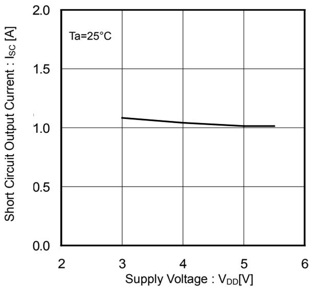
Figure 13. Short Circuit Output Current vs Supply Voltage
