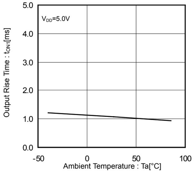
Figure 18. Output Rise Time vs Ambient Temperature
