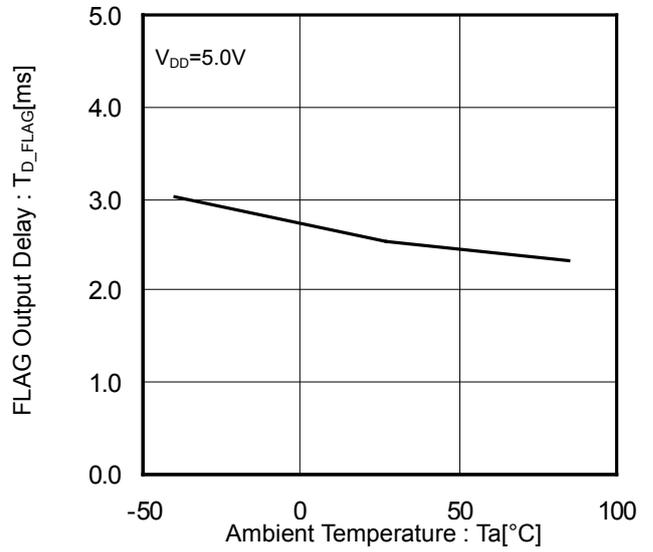
Figure 16. FLAG Output Delay vs Ambient Temperature
