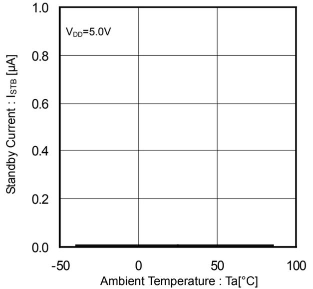
Figure 6. Standby Current vs Ambient Temperature (CTRL Disable)
