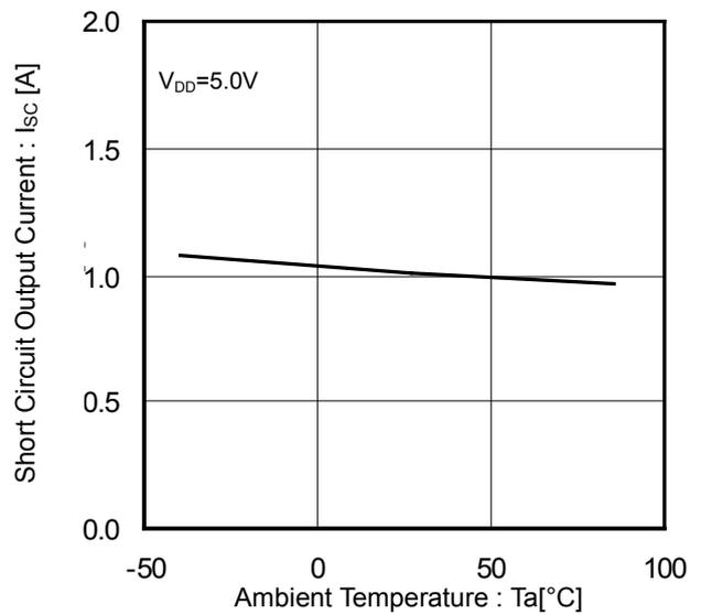
Figure 14. Short Circuit Output Current vs Ambient Temperature
