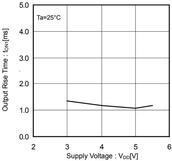
Figure 17. Output Rise Time vs Supply Voltage
