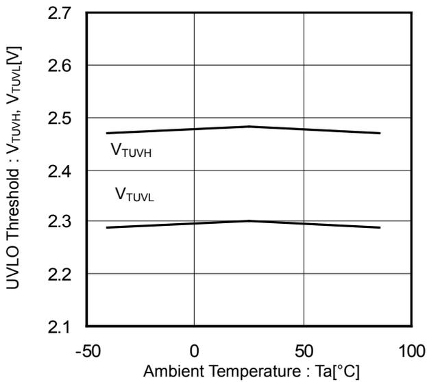
Figure 25. UVLO Threshold Voltage vs Ambient Temperature
