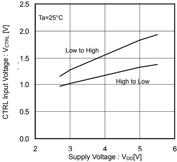
Figure 7. CTRL Input Voltage vs Supply Voltage
