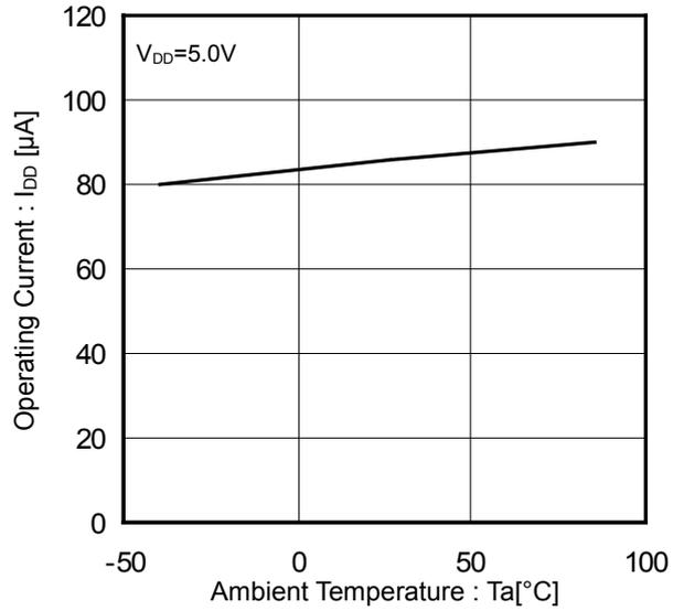
Figure 4. Operating Current vs Ambient Temperature (CTRL Enable)
