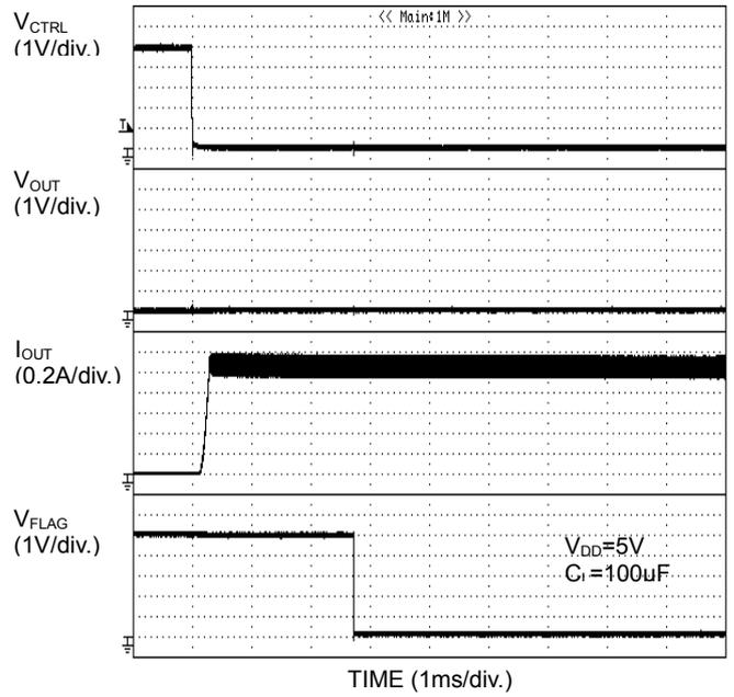
Figure 32. Over-Current Response Enable to Short Circuit
