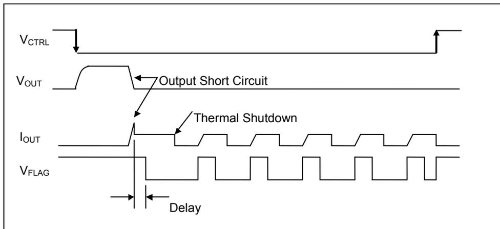
Figure 37. Over-Current Detection, Thermal Shutdown Timing Diagram
