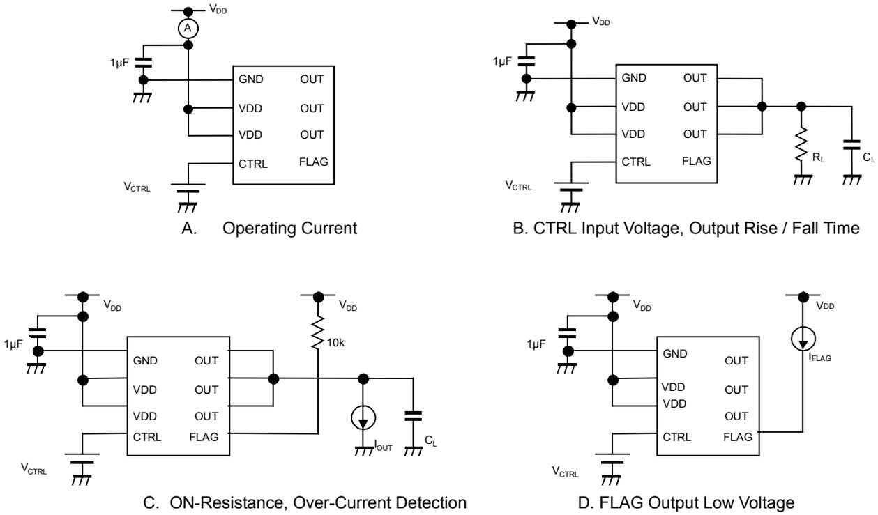
Figure 1. Measurement Circuit
