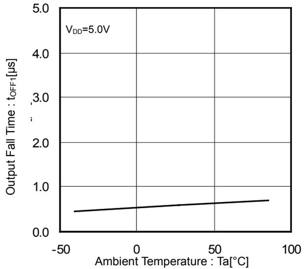
Figure 22. Output Fall Time vs Ambient Temperature
