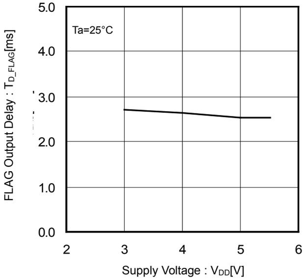
Figure 15. FLAG Output Delay vs Supply Voltage
