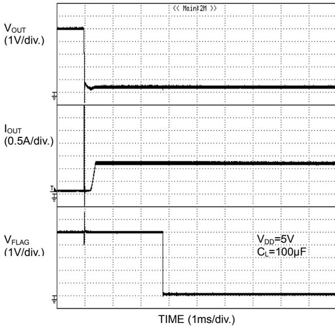
Figure 33. Over-Current Response Output Short Circuit at Enable
