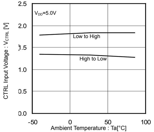
Figure 8. CTRL Input Voltage vs Ambient Temperature
