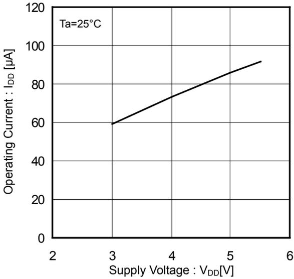
Figure 3. Operating Current vs Supply Voltage (CTRL Enable)
