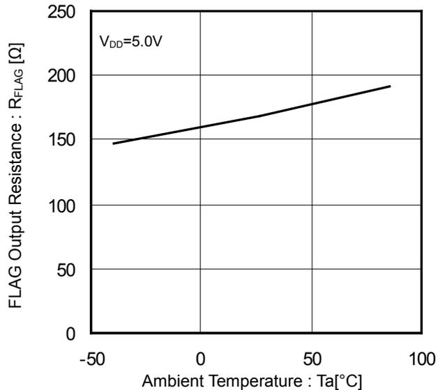
Figure 10. FLAG Output Resistance vs Ambient Temperature
