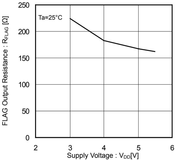
Figure 9. FLAG Output Resistance vs Supply Voltage
