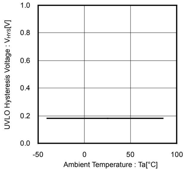
Figure 26. UVLO Hysteresis Voltage vs Ambient Temperature
