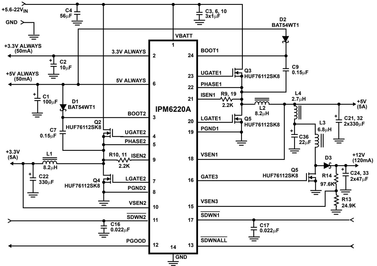
FIGURE 11. APPLICATIONS CIRCUIT
