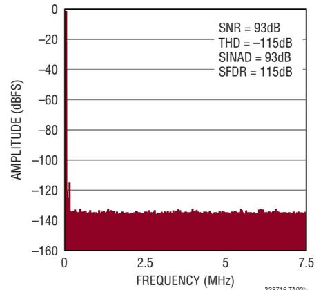
128k Point FFT,  $f_{\text{SAMPL}} = 15\text{Mps}$ ,  $f_{\text{IN}} = 50\text{kHz}$
