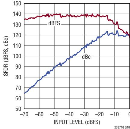
**SFDR vs Input Level,  $f_{IN} = 1\text{MHz}$**
