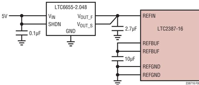
Figure 8. Using the LTC6655-2.048 as an External Reference
