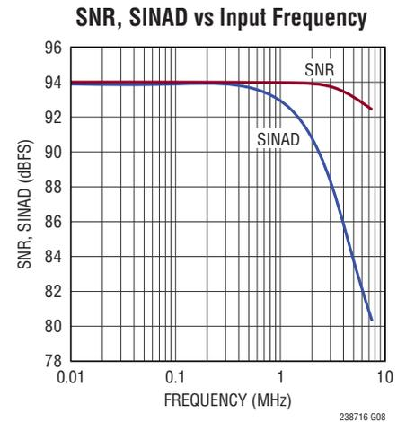
**TYPICAL PERFORMANCE CHARACTERISTICS**  $T_A = 25^\circ\text{C}$ ,  $V_{DD} = 5\text{V}$ ,  $V_{DDL} = 2.5\text{V}$ ,  $OV_{DD} = 2.5\text{V}$ ,
