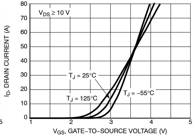
Figure 2. Transfer Characteristics
