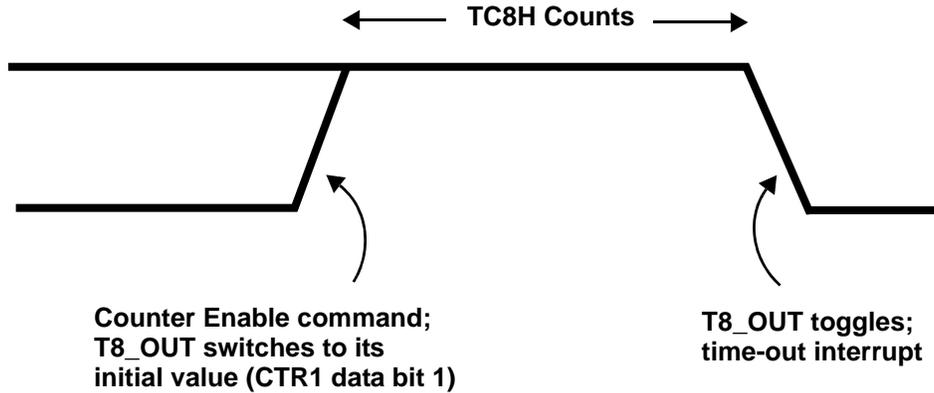
Figure 30. T8\_OUT in SINGLE-PASS Mode
