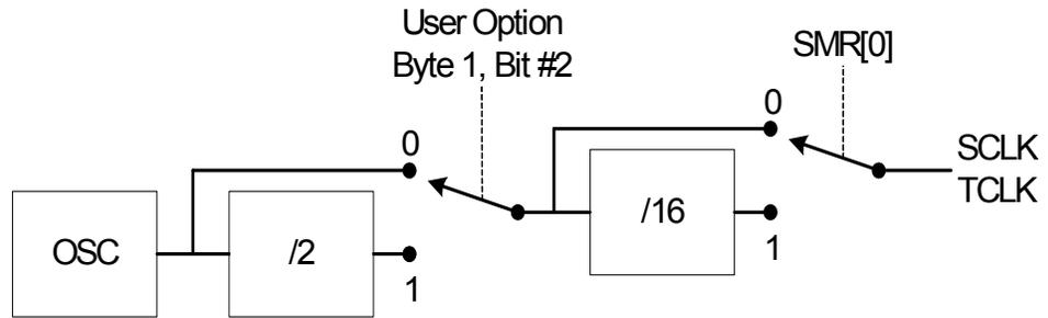
Figure 42. SCLK/TCLK Circuit
