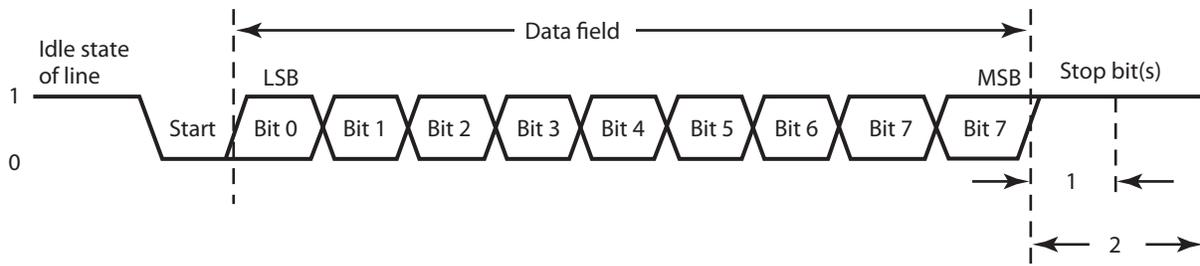
**Figure 24. UART Asynchronous Data Format with Parity**
