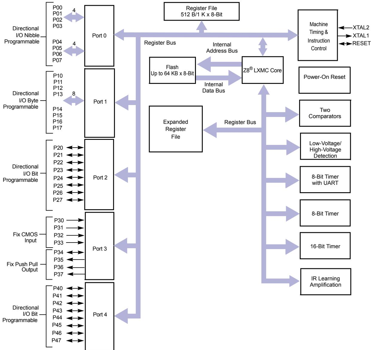
Figure 1. ZLF645 Flash MCU Functional Block Diagram
