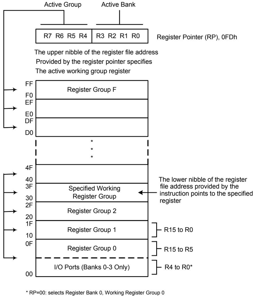
**Figure 14. Register Pointer—Detail**
