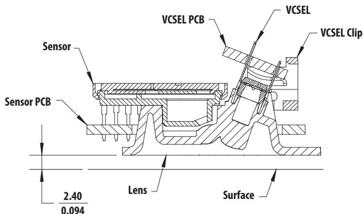
Figure 10. Distance from lens reference plane to surface
