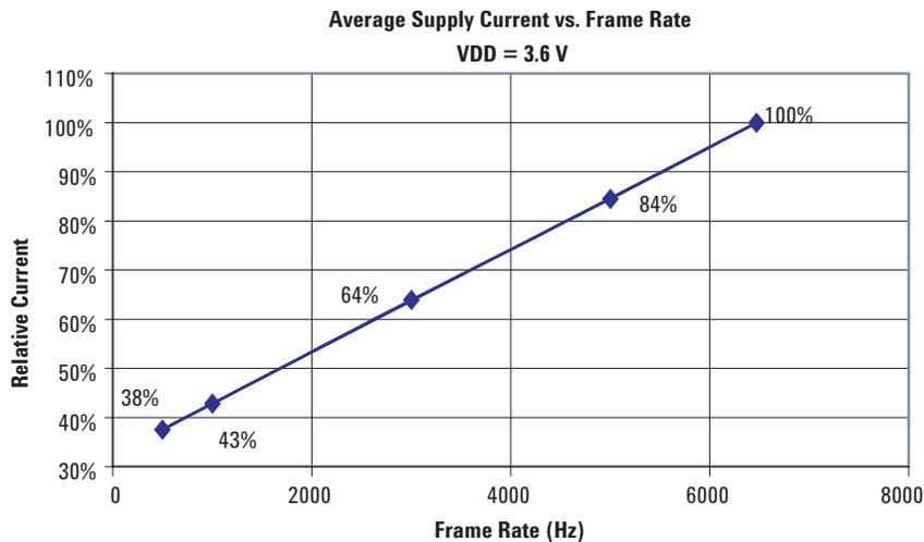
Figure 14. Average Supply Current vs. Frame Rate
