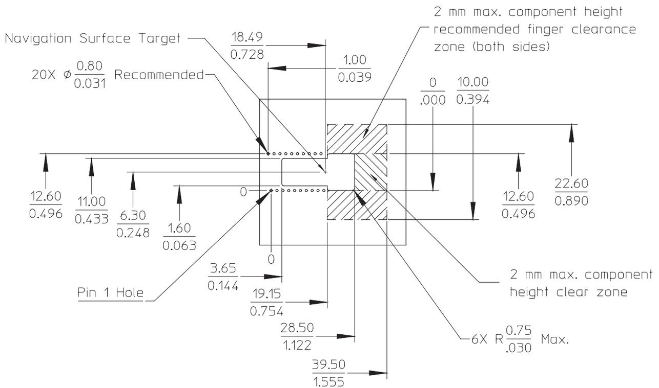
Figure 5. Recommended PCB mechanical cutouts and spacing
