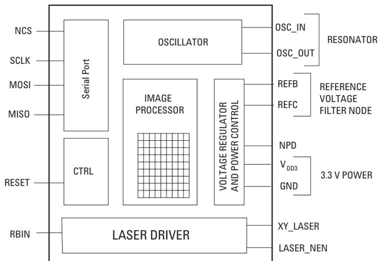
Figure 8. Block diagram of ADNS-6000 optical mouse sensor
