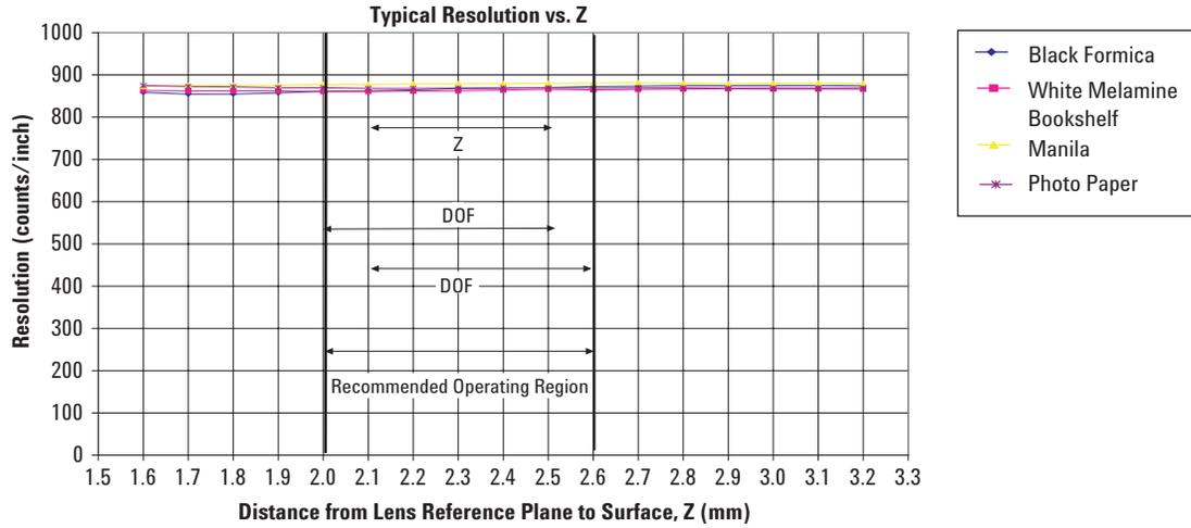
Figure 12. Mean Resolution vs. Z at 800cpi
