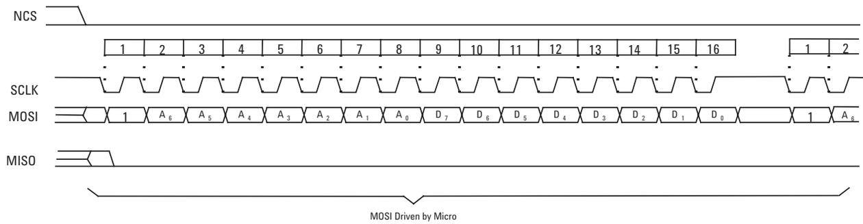
Figure 17. Write Operation
