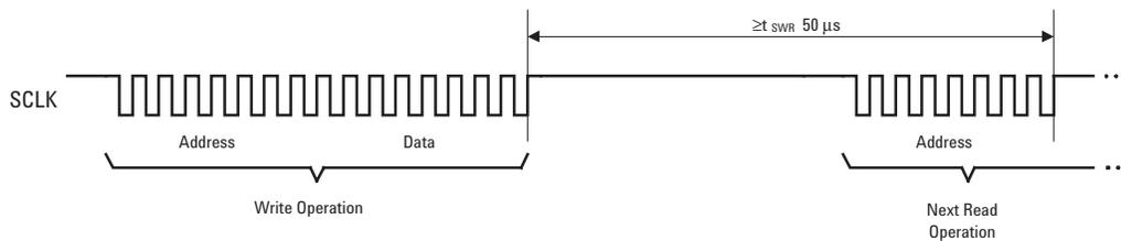
Figure 21. Timing between write and read commands
