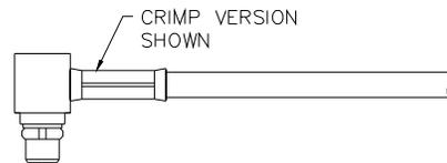
8. PRESS INSULATOR AND CAP INTO CONNECTOR BODY AS SHOWN.
