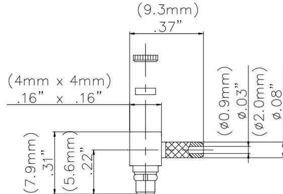
Snap-on coupling and micro-miniature size for fast connect and disconnect where space is limited
