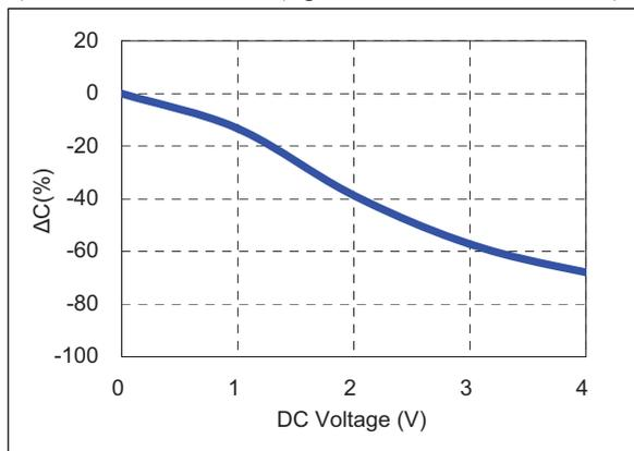
4) Bias TCC characteristics (Agilent 4284A, 120Hz, 0.5Vrms, 2Vdc)
