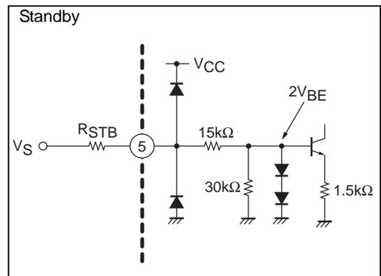
Note that the standby pin (pin 5) incorporates the anti-electrostatic diode, allowing the current to flow through the diode when the potential of  $V_{CC}$  pin 7 decreases below that of pin 5.
