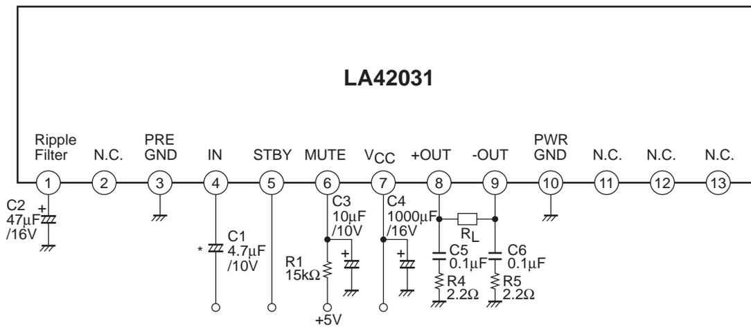
\* LA42031 employs the zero-bias type input circuit, with the input pin potential being nearly zero (about 0.01V). Accordingly, the polarity must be determined according to the DC potential of a circuit connected to the previous stage of LA42031.
