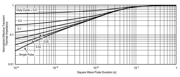
Normalized Thermal Transient Impedance, Junction-to-Foot
