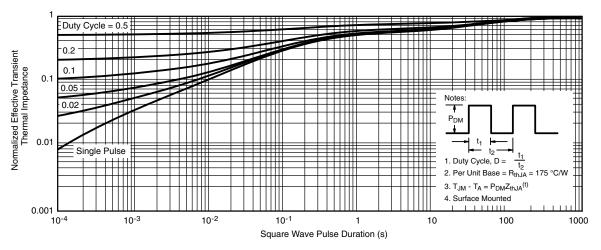
Normalized Thermal Transient Impedance, Junction-to-Ambient
