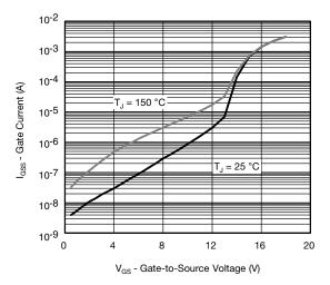
Gate Current vs. Gate-Source Voltage
