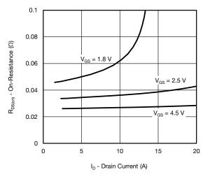
On-Resistance vs. Drain Current
