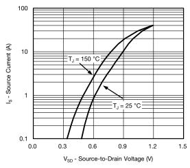
Soure-Drain Diode Forward Voltage
