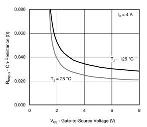
On-Resistance vs. Gate-to-Source Voltage
