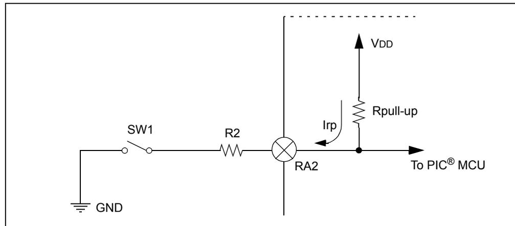
As seen in [Figure 3-12](#), by enabling the weak pull-up on a pin, the pin will always read a '1' if no other external circuitry is connected to RA2. In this demo, there is a resistor connected to the switch, which is then connected to ground. When the switch is pressed, the voltage on RA2 is no longer VDD, but rather close to 0V, or ground.
