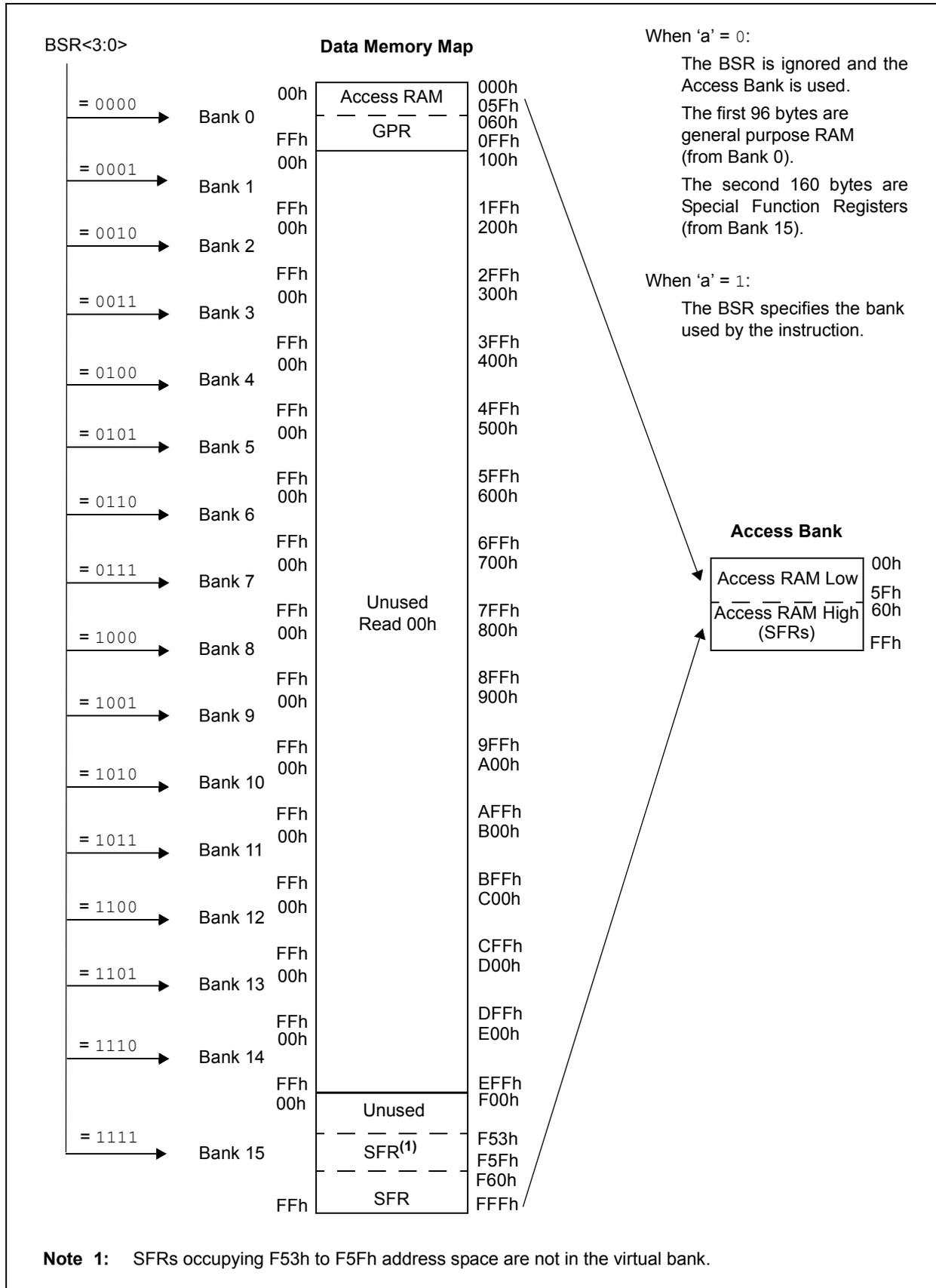
**FIGURE 2-11: PIC18F14K22 SPECIAL FUNCTION REGISTER MAP – ALL OF THESE ARE IN BANK 15 WHICH IS INCLUDED IN THE “ACCESS RAM”**
