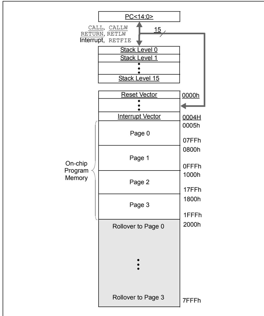
PIC18 devices are capable of addressing a 2-Mbyte program memory space, as seen in [Figure 2-7](#). PIC18 devices also have two interrupt vectors, whereas the enhanced PIC devices only have one. A stark difference is that the PIC18 has no concept of pages, whereas the enhanced core has its program memory split into different pages.
