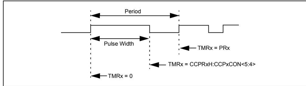
The PWM period is specified by the PRx register. Timer 2/4/6 is used to count up to the value in CCPRxH combined with two LSbs in CCPxCON. CCPRxL is used to load CCPRxH. One can think of CCPRxL as a buffer which can be read or written to, but CCPRxH is read-only. When the timer is equal to PRx, the following three events occur on the next increment cycle:
