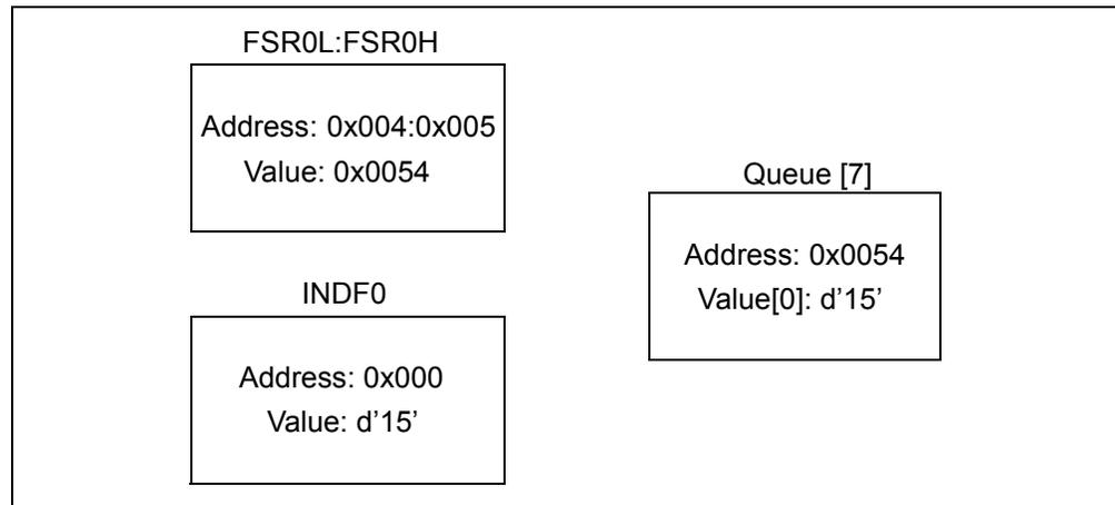
After `FilterInit` is called, the FSR0 register is pointing towards the first byte in queue. The INDF0 register can now be read/written to. Any affects on the INDF0 register will affect the value at the assigned address in the FSR0 register. An increment of FSR0 will point to the next byte in the Queue register. In this case, it is the second ADC reading.
