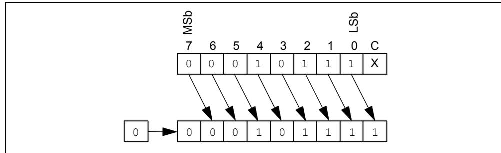
**FIGURE 3-2: ROTATE RIGHT THROUGH CARRY**
