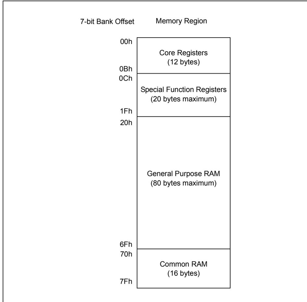
Addresses 70h-7Fh are shared by all of the banks. This is useful for storing a few bytes of RAM without the need to switch banks each time the byte is used. [Figure 2-9](#) shows the first eight banks on the PIC16F1829. Notice how the top 12 core registers are accessible from every bank, as are the 16 bytes of common RAM.
