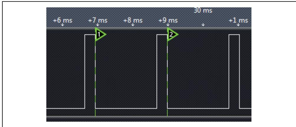
Figure 3-10 shows when the dial is turned 30% clockwise. Notice how the pulse width is greater than that shown in Figure 3-9, and that the frequency did not change.
