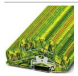
Double-level terminal block, Cross section: 0.14 mm<sup>2</sup> - 4 mm<sup>2</sup>, AWG: 26 - 12, Connection type: Push-in connection, Width: 5.2 mm, Color: green-yellow, Mounting type: NS 35/7,5, NS 35/15
