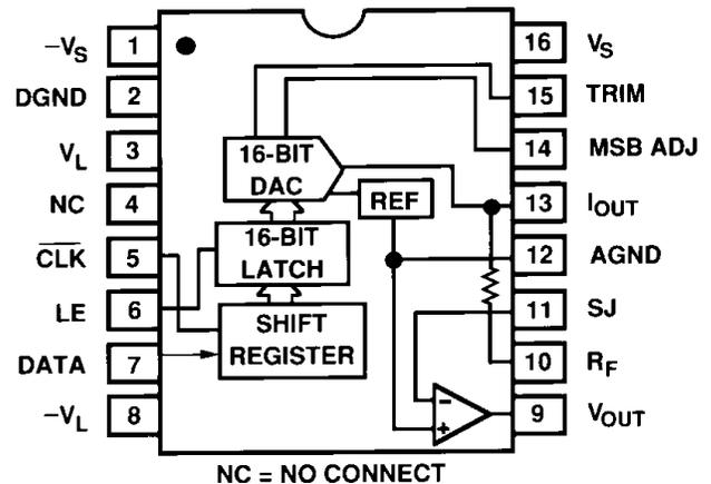
The serial interface consists of bit clock, data, and latch enable inputs. The twos-complement data word is clocked MSB first on falling clock edges into the serial-to-parallel converter, consistent with the serial protocols of popular DSP processors. The input clock can support data transfers up to 12.5 MHz. The falling edge of latch enable updates the internal DAC input register at the sample rate with the sixteen bits most recently clocked into the serial input register.
