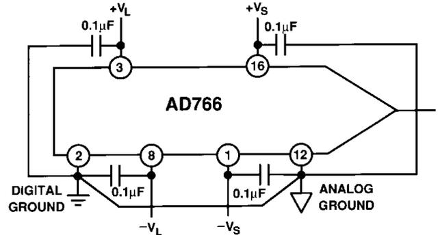
Figure 5. Recommended Circuit Schematic
