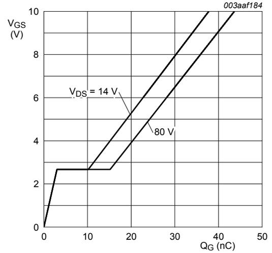
$T_j = 25\text{ }^\circ\text{C}; I_D = 10\text{ A}$
