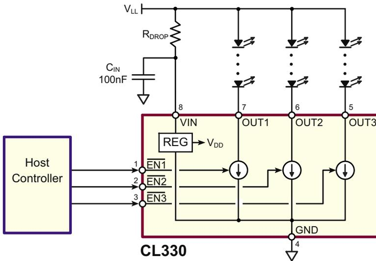
$$R_{DROP} < \frac{V_{LL(MIN)} - 6.5V}{2.3mA}$$
