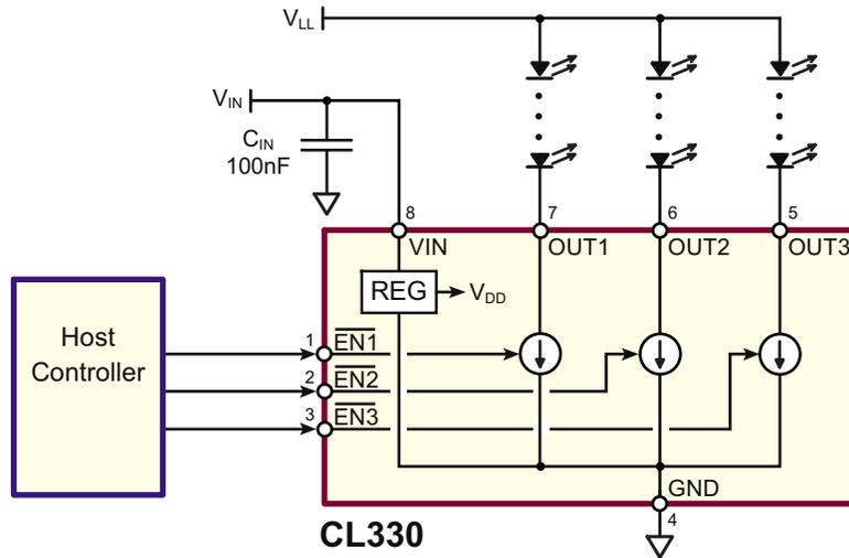
CL330 power dissipation may be lowered by supplying the CL330 from a voltage source ( $V_{IN}$ ) that is lower in voltage than the LED supply ( $V_{LL}$ ).
