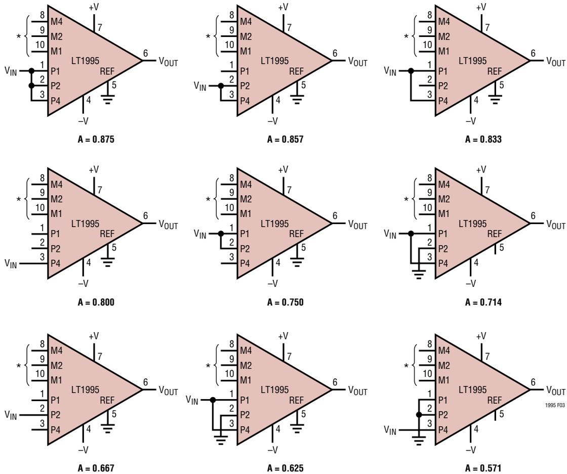
\*CONFIGURE M INPUTS FOR DESIRED G PARAMETER; REFER TO FIGURE 2 FOR CONNECTIONS
