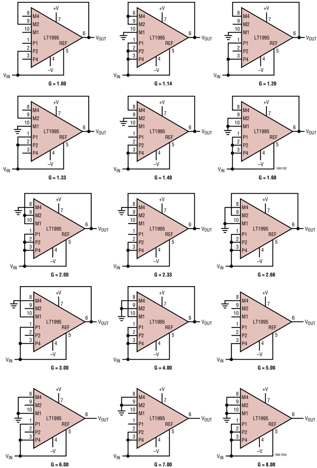
Figure 2. Noninverting Buffer Amplifier Configurations (Hi-Z Input)
