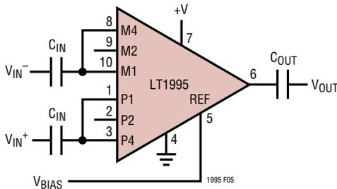
Figure 5. AC-Coupled Difference Amplifier General Configuration (G = 5 Example)
