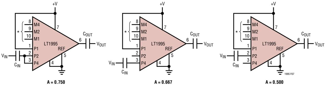
\* CONFIGURE M INPUTS FOR DESIRED G PARAMETER; REFER TO FIGURE 2 FOR CONNECTIONS. ANY M INPUTS SHOWN GROUNDING IN FIGURE 2 SHOULD INSTEAD BE CAPACITIVELY COUPLED TO GROUND
