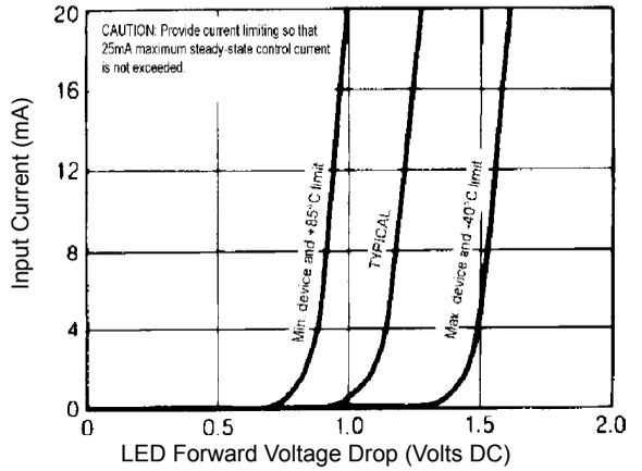
Figure 6. Input Characteristics
