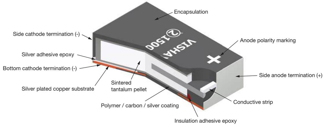
**TANTALUM CAPACITOR WITH POLYMER CATHODE TYPE T54 / T59**
