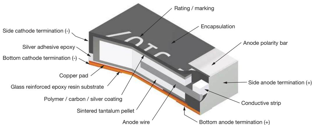
**TANTALUM CAPACITOR WITH POLYMER CATHODE TYPE T52**
