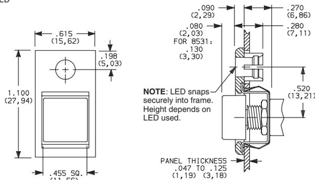
**NOTE:** LED snaps securely into frame. Height depends on LED used.
