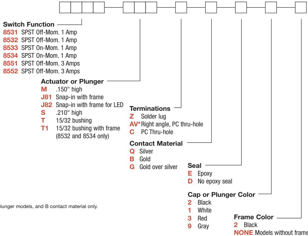
\* Available with M or S plunger models, and B contact material only.
