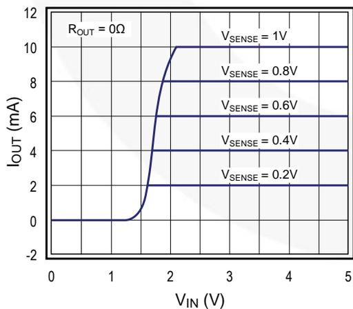
Figure 8. Transfer Characteristics
