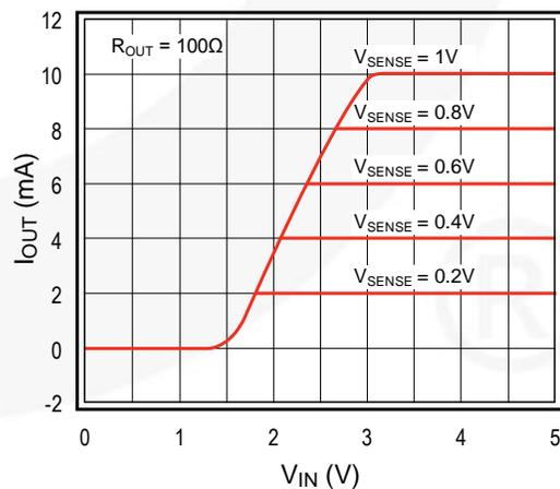
Figure 9. Transfer Characteristics
