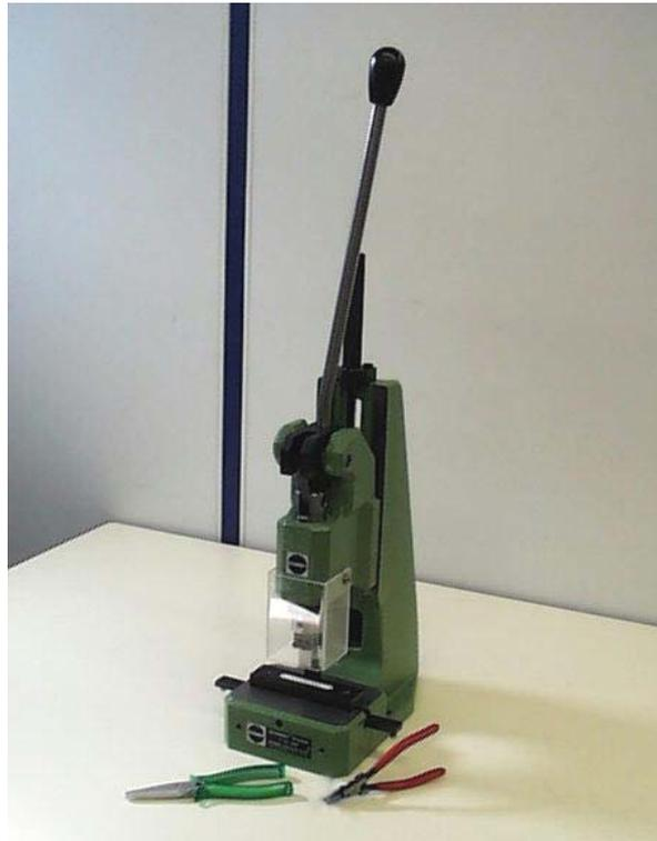
**Figure 17 -- Connector Removal tooling HM2Y350**
