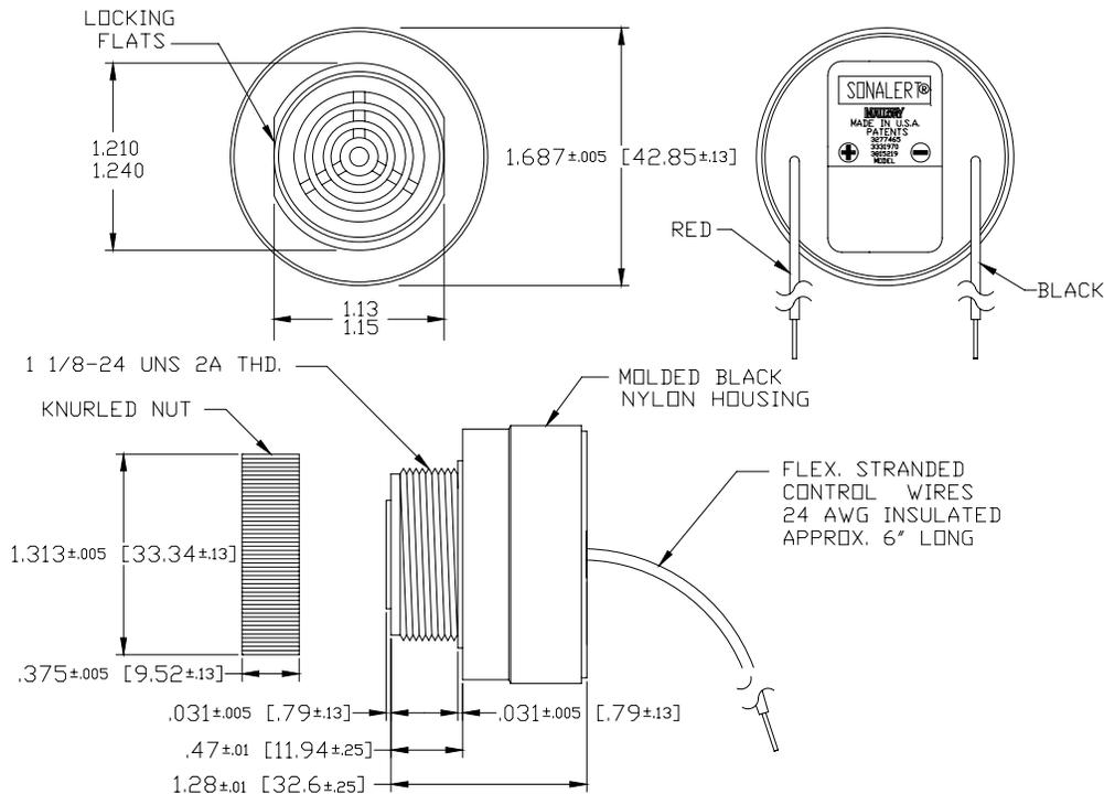
NOTE: MOUNTING- REMOVE BLACK PLASTIC NUT AND INSERT THREADED FRONT THROUGH 1.25" HOLE PUNCHED IN PANEL, IF ORIENTATION IS NEEDED, NOTE LOCKING FLATS ON DRAWING. SCREW NUT BACK ON. DO NOT OVERTIGHTEN.
