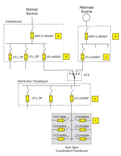
Selective coordination is as simple as maintaining amp rating ratios of 2:1 or greater between all CUBEFuse and Low-Peak fuses in a circuit. For other fuse types see published ratios.
