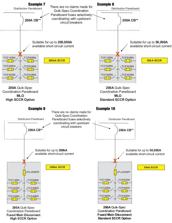
\*\* Circuit breaker interrupting ratings must be equal to or greater than available short-circuit current at their line-side per NEC® 110.9.
