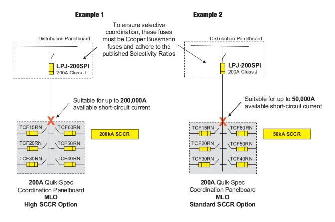
Quik-Spec™ Coordination Panelboard Short-Circuit Current Ratings with Upstream Fuses (600Vac or less system)
