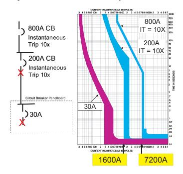
Figure 6 – Molded-Case & Power Circuit Breaker System
