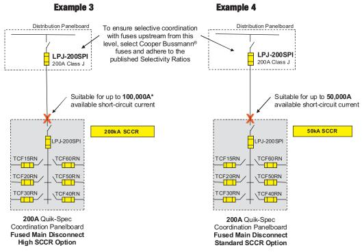
Note the upstream 200A fuses do not have to selectively coordinate with the 200A panelboard main fuses because if both open, no additional parts of the electrical system would be shut down unnecessarily. See NEC<sup>®</sup> 700.27 and 701.18 exceptions.
