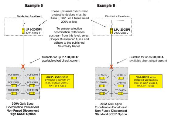
Quik-Spec™ Coordination Panelboard Short-Circuit Current Ratings with Upstream Circuit Breakers (600Vac or less system)
